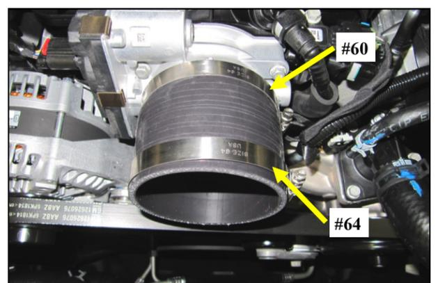
6. Slide the Coupler with a #60 and #64 clamp onto the throttle body as shown.
