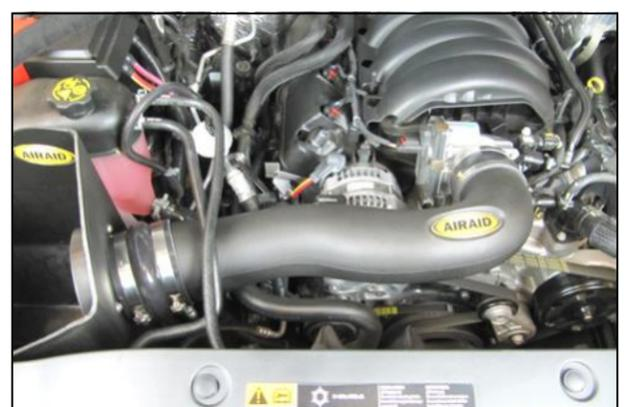
9. Install the Airaid Intake Tube into the Hump Hose and couplers. Adjust for fit and tighten all four Hose Clamps.
