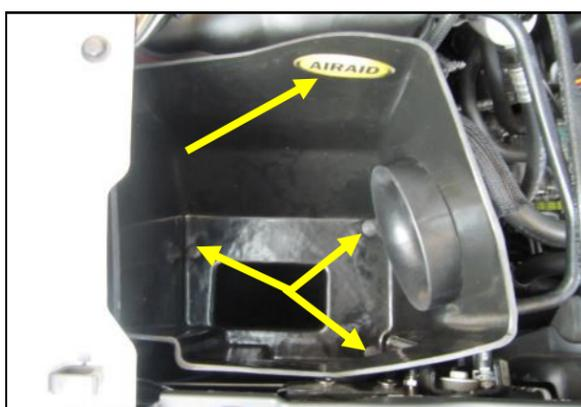
5. Slide the Airbox assembly into the inner fender area and secure it using 3 of the OEM bolts removed in step 3. Apply the Airaid Decal inside of the Airbox as shown.
