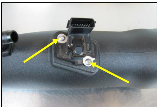
7. Transfer the Mass Air Flow sensor from the factory airbox into the Airaid Intake Tube. Secure the sensor using the two 8-32 Button Head Screws.
