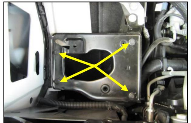
3. Remove the 4 bolts in the airbox mounting tray and set them aside. They will be reused in step 5. Remove the Tray, it will not be re-used.
