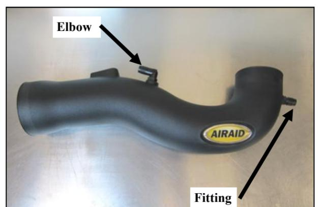
6. Install the Barbed Fitting and Elbow into the Airaid Intake Tube. Apply the Airaid Decal onto the Tube as shown.
