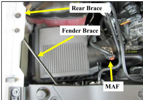
2. Using an open end wrench, remove the passenger side fender brace and set it aside. For ease of installation, remove the rear brace bolt and set it aside. Unplug the Mass Air Flow sensor, or MAF and unanchor it from the airbox. Unseat the airbox from its mounting grommets and remove the factory airbox.
