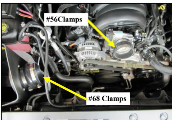
8. Slide the Hump Hose with the #68 Hose Clamps onto the Filter adapter and the coupler and the #56 Clamps onto the throttle body. Leave the clamps loose for now.
