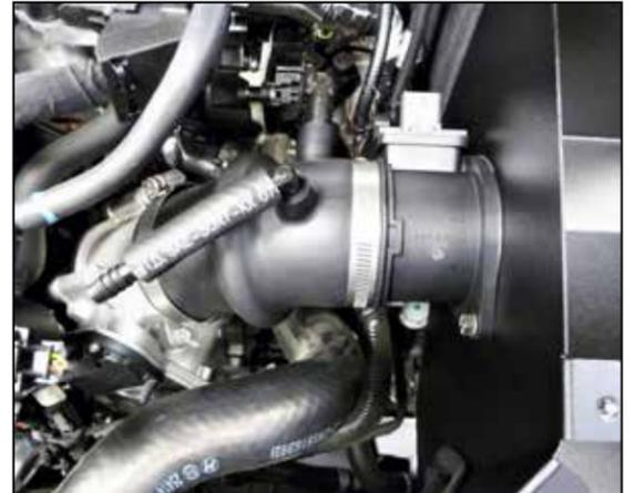
14. Install the hose/maf housing assembly onto the throttle body and into the heat shield. Adjust the maf housing so the holes line up and secure with the provided hardware. Adjust the hose for best fit and then secure with the provided hose clamps.
