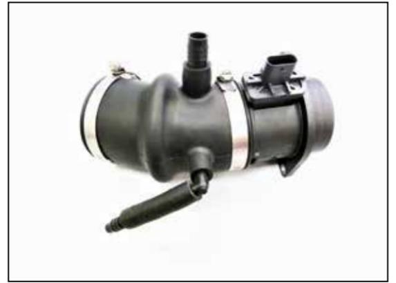
13. Install the factory mass air sensor into the AEM hose as shown but don't tighten the clamp.
