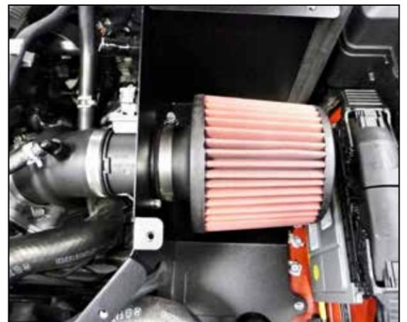
16. Install the AEM air filter onto the mass air sensor and secure with the provided hose clamp.
