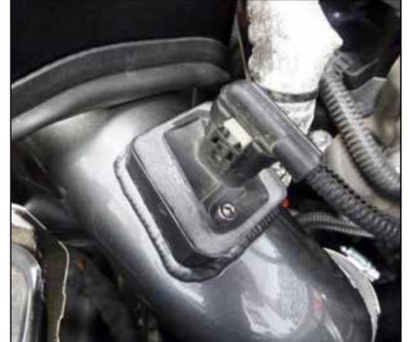
14. Connect the mass air sensor electrical connection.
