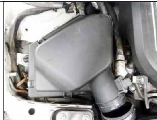
3. Lift air filter housing straight up and remove it from the vehicle.
