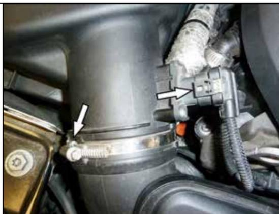
2. Loosen the hose clamp that secures the factory intake tube to the air filter housing and then separate the tube from the housing. Disconnect the mass air sensor electrical connection.
