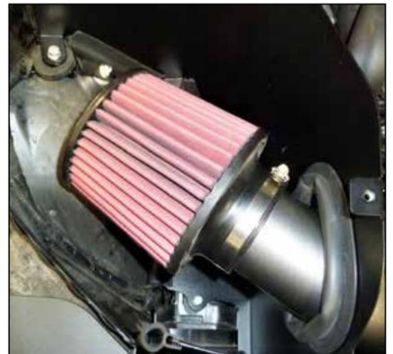
14. Install the air filter onto the intake tube and secure with the provided hose clamp. Adjust the tube for best fit and then secure the hose clamp.
