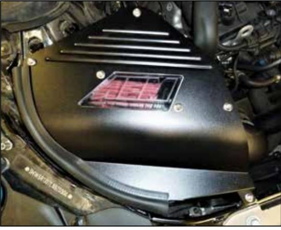
16. Install the lid onto the heat shield and secure with the provided hardware.
