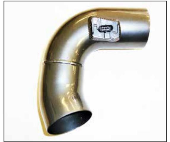
12. Remove the mass air sensor from the factory air filter housing and install it into the AEM intake tube and secure with the provided hardware.
