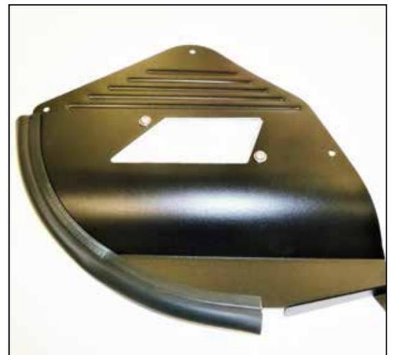
15. Install the AEM window into the lid and then install the edge trim as shown.
