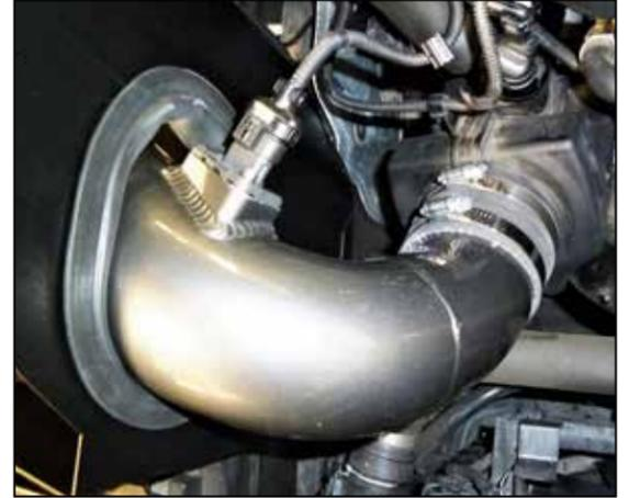
13. Install the intake tube through the hole in the heat shield and then into the coupler. Do not secure the hose clamp at this time. Connect the mass air sensor electrical connection.
