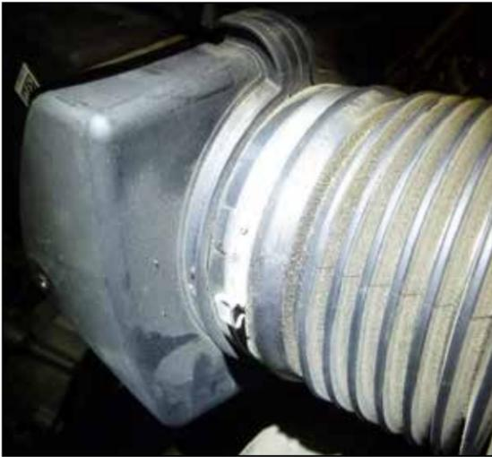
6. Cut the one-time use clamp that secures the intake hose to the intake plenum and then remove the intake tube from the vehicle.
