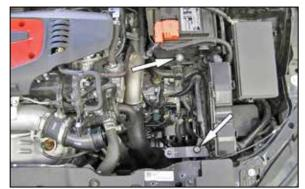
5. Install the two rubber mounted studs to the air filter housing mounting locations. Remove the plastic harness holder from the mass air sensor wiring harness and then install the provided split loom harness cover. Tape the ends of the harness cover with electrical tape.
