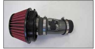
12. Install the AEM<sup>®</sup> air filter onto the filter adapter
