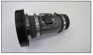
11. Install the filter adapter assembly onto the AEM<sup>®</sup> intake tube and secure with the provided hose clamp. Install coupler (084034) onto the AEM<sup>®</sup> intake tube and secure with the provided hose clamp.
