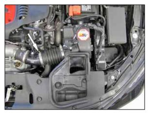
3. Release the clips that secure the upper air filter housing, loosen the hose clamp that secures the intake tube to the turbo inlet and then remove the upper air filter housing and intake tube from the vehicle.
