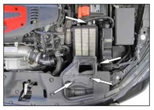
4. Remove the four bolts that secure the lower air filter housing and fresh air scoop to the vehicle and remove the complete assembly from the vehicle. **NOTE: AEM recommends that customers do not discard factory air intake.**
