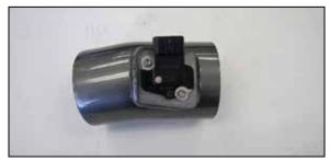
9. Remove the mass air sensor from the factory housing and install into the AEM<sup>®</sup> intake tube and secure with the provided hardware.
