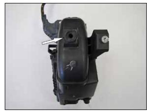
6. Remove the factory air filter housing mounting grommet from the factory housing.
