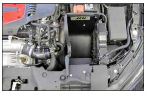
8. Set the heat shield into position on the rubber mounted studs and mounting stud. Secure the heat shield with the provided hardware.
