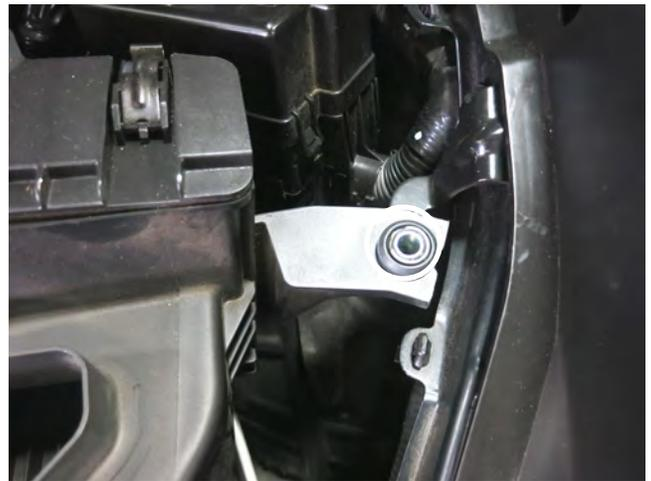
d. Remove the M6 bolt in the location shown above.
