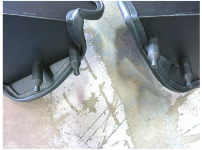
f. Install the post mounts to the bottom of the heat shields.
