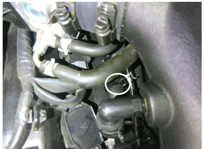
j. Reposition the spring clamp onto the breather hose (driver side pictured).
