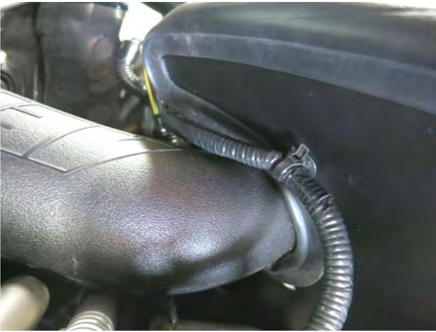
m. Route the MAF harness above the intake tube and clip it into the provision on the heat shield. Repeat for other side.
