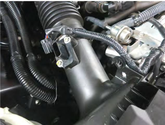
c. Unplug the Mass Air Flow (MAF) sensor harness and unclip it from the air box. Repeat for other side.
