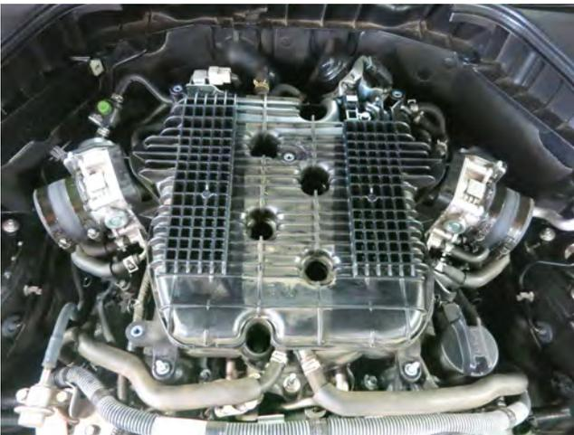
c. Install the [2] couplers along with [4] hose clamps onto the throttle bodies as shown. Tighten the hose clamps on the throttle body side at this time.
