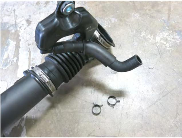
k. Remove the [2] spring clamps from the breather hose (passenger side pictured). Do not discard any factory components or hardware removed thus far.
