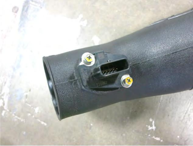
a. Install the MAF sensors into both AEM intake tubes.
