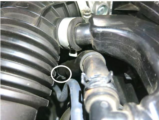
g. Use pliers to release the spring clamp shown above (passenger side pictured).
