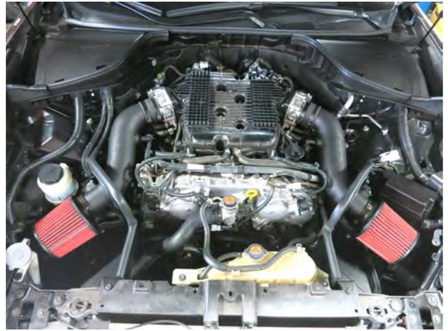
l. Install the AEM filters. Orient them for best fit. Then tighten the hose clamps on the throttle body couplers to fully secure the intake tubes.
