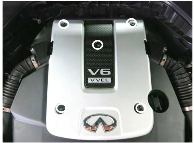
b. Use a 10mm socket and ratchet to remove the [2] nuts and [3] bolts holding the engine cover. Remove the cover.
