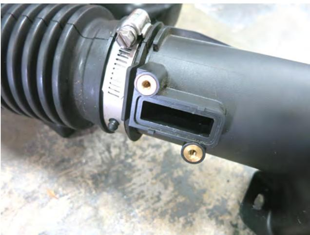
i. Remove the MAF sensor from the intake tube. Repeat for other intake tube.
