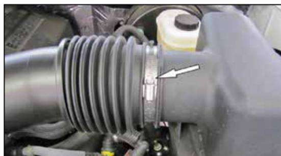
3. Loosen the hose clamp that secures the factory intake tube to the upper air filter housing.
