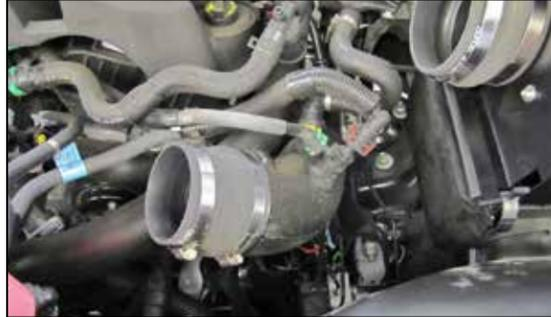
13. Install the provided coupler (08497) onto the driver's side turbo inlet tube and secure with the provided hose clamp.
