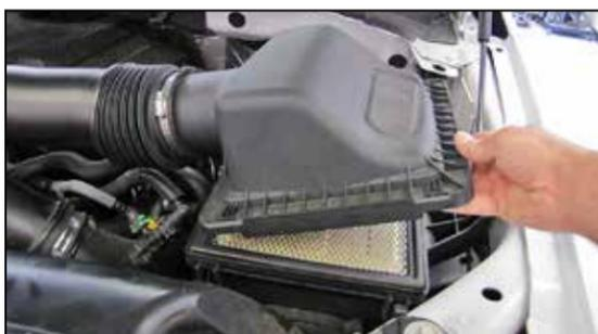
4. Release the locking clips that secure the upper air filter housing to the lower housing, then lift the upper housing and remove it from the vehicle. Remove the factory air filter from the vehicle.
