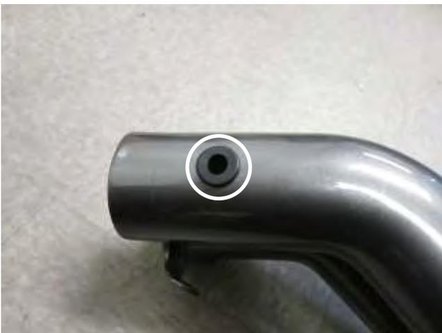
a. Install the provided grommet into the AEM<sup>®</sup> intake tube.
