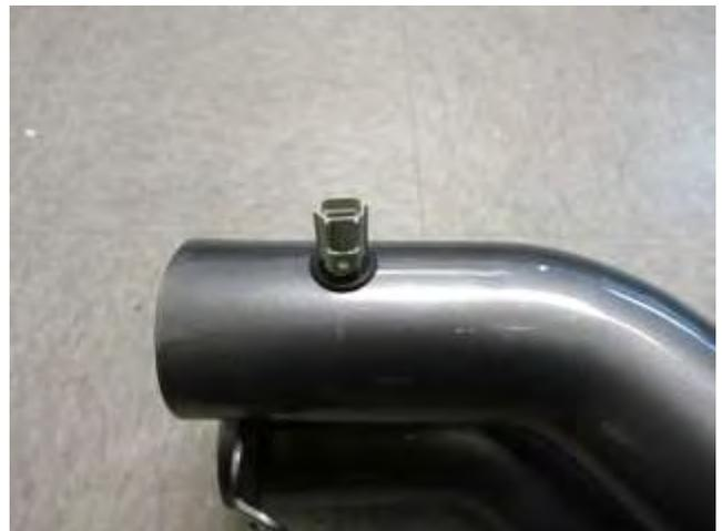
b. Install the air temperature sensor that was removed in step 2g into the AEM<sup>®</sup> intake tube.
