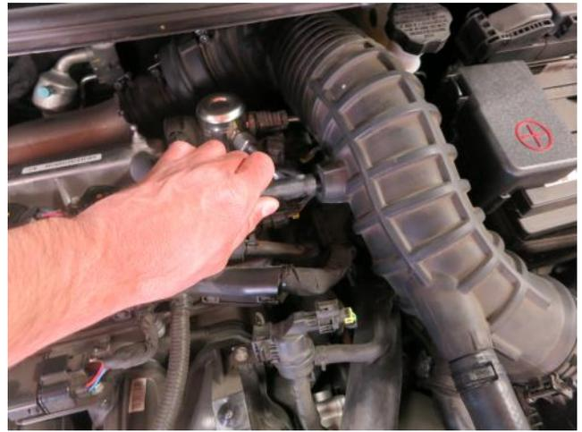
b. Remove the PCV hose from the stock air box tube by using a set of pliers to release the spring clamp.
