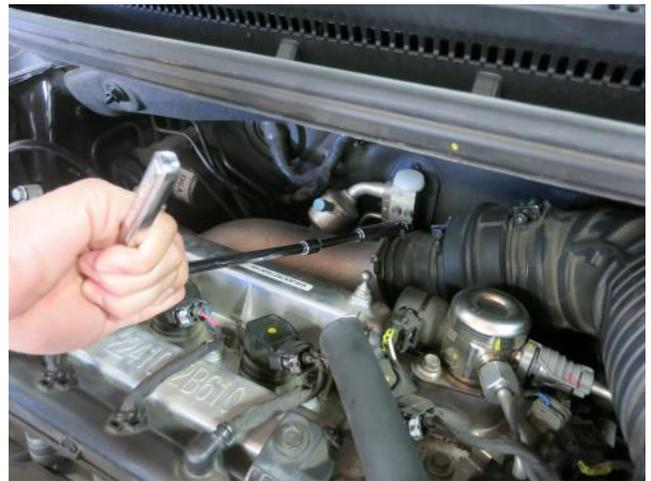
d. Loosen the band clamp with a 10mm socket and ratchet. **DO NOT REMOVE INTAKE HOSE UNTIL STEP 2e IS COMPLETED.**
