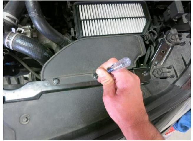
f. Remove the 2 clips holding the air scoop with a screwdriver by depressing the center pin.
