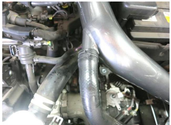
n. Reinstall the recirculation hose to the intake tube using the stock spring clamp.
