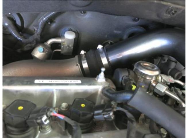
l. Properly align the intake to make sure there is clearance, then tighten the 2 band clamps with an 8mm nut driver. Torque spec: 30in-lb.
