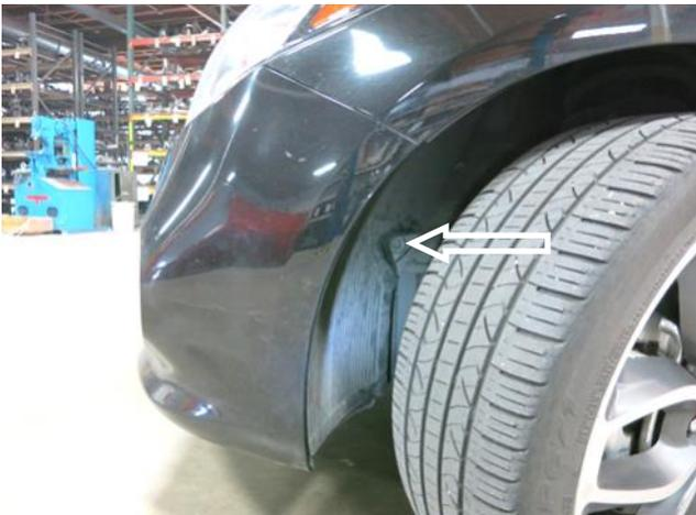
g. Turn the steering wheel to the left and remove the fender liner clip by using a #2 Phillip screwdriver.
