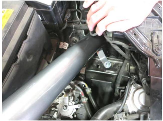
f. Attach the intake tube to the rubber mount. DO NOT TIGHTEN THE BAND CLAMPS UNTIL FILTER IS INSTALLED.
