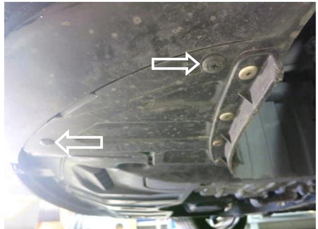
h. Remove the 2 fender liner clips by using a #2 phillips screwdriver.
