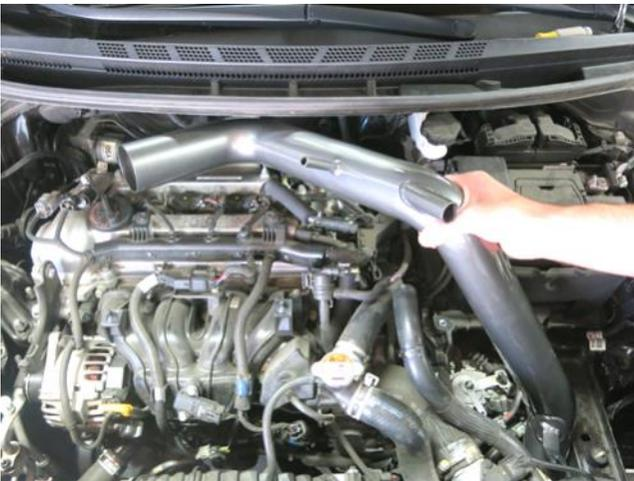
c. Install the AEM intake tube by dropping the filter end inside the frame rail first, then swing the throttle body side in towards the fire wall.
