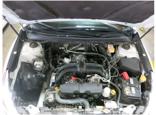
f. Remove the stock intake system from the vehicle. **Do not discard any factory intake components.**
