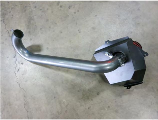
e. Secure the intake tube to the rubber mount by tightening the nut with a 10mm socket and ratchet.
