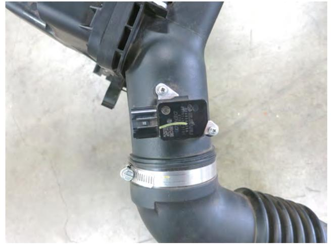
h. Remove the two screws that secure the MAF sensor. Then, set the MAF sensor aside for later installation.
