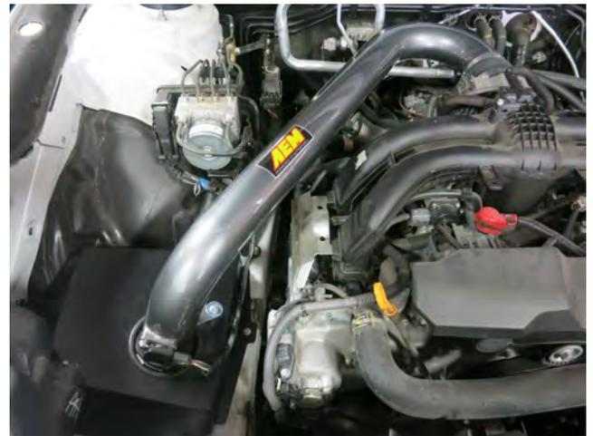
j. Reconnect the MAF sensor plug to the sensor.
