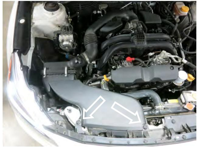
b. Remove the 2 clips that secure the intake scoop.
