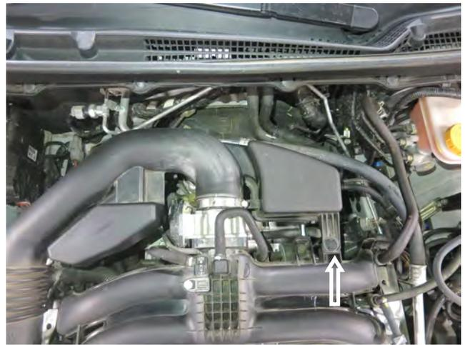
d. Remove the clip that secures the resonator. Also, loosen the hose clamp on the intake tube with an 8mm socket driver.
