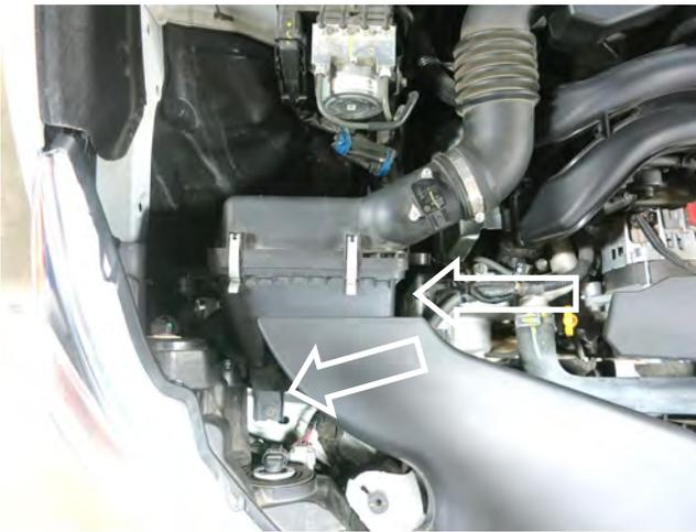
c. Remove the 2 bolts that secure the air box with a 10mm socket, 1/4" extension, and ratchet. Then pull up on the air box to remove from the rubber grommets.
