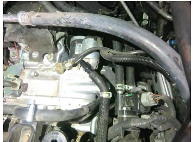
h. Install the plastic connector to the vent hose as shown.
