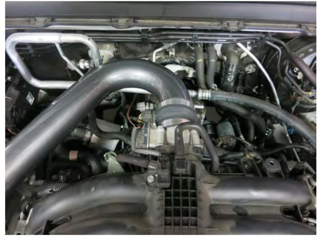
f. Install the AEM intake tube into the coupler. DO NOT FULLY TIGHTEN THE HOSE CLAMP AT THIS TIME.
