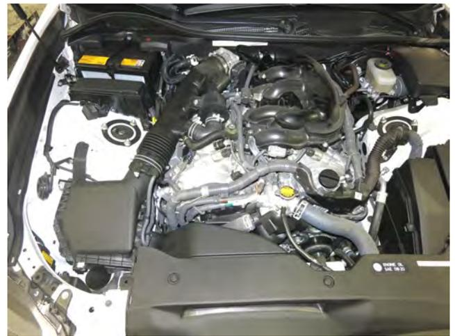
b. Remove the plastic engine cover by pulling up gently to release the rubber grommets.
