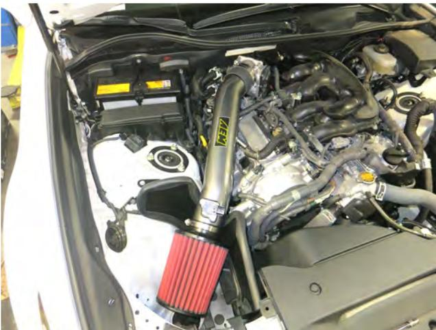
g. Install the AEM intake tube into the coupler first, then lower the bracket into the gap between the washer installed in step 3c and the engine. Torque the hose clamp to 30 in-lb at this time.
