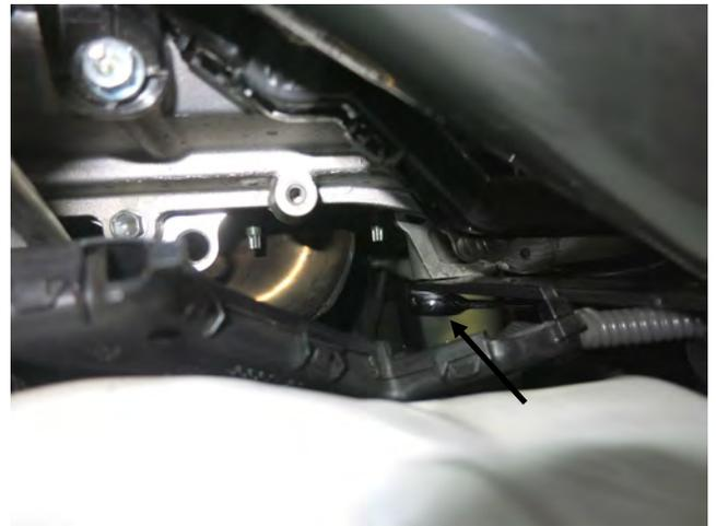
h. Tighten the bracket using a 12mm wrench. This area can be accessed from the front of the engine. This picture is as seen from the shock tower looking downward.
