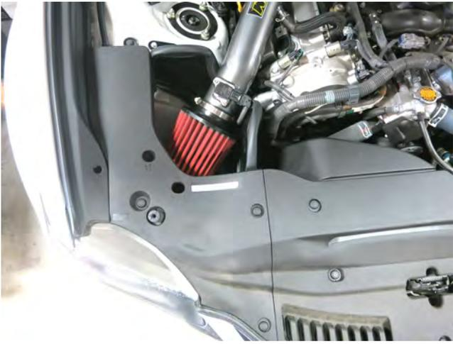
k. Reinstall the plastic shroud over the heat shield and filter using the plastic rivets removed in step 2a. Push the rivets into the popped-up position before installing them, then push them flush to secure.
