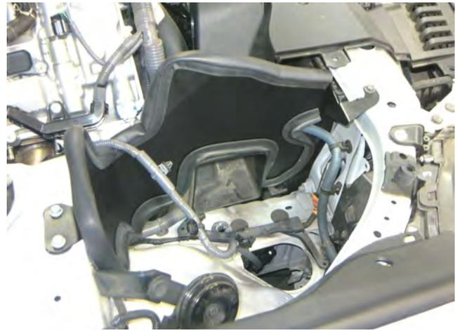
f. Install the heat shield as shown using the two provided bolts and the core support bolt removed earlier. The scoop position may need adjusting during installation.
