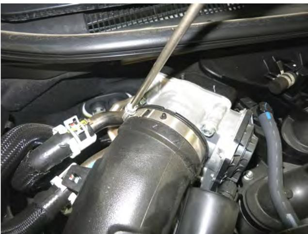
g. Loosen the factory hose clamp at the throttle body and remove the end of the factory tube from the throttle body.
