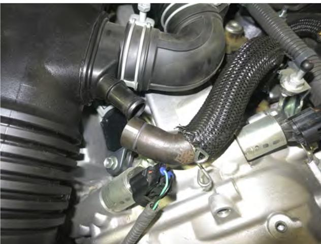
c. Disconnect the vent hose by pinching the spring clamp while pulling it from the factory tube.
