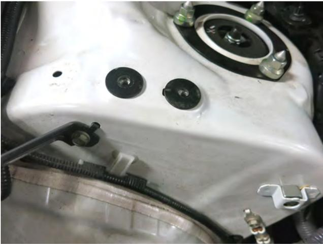
e. Place the two included rubber washers over the mounting holes on the shock tower.
