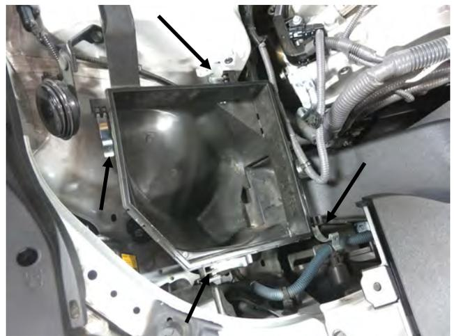
h. Release the 4 latches on the air box securing the lid and factory tube. Remove the lid, factory tube, and filter from the engine bay.
