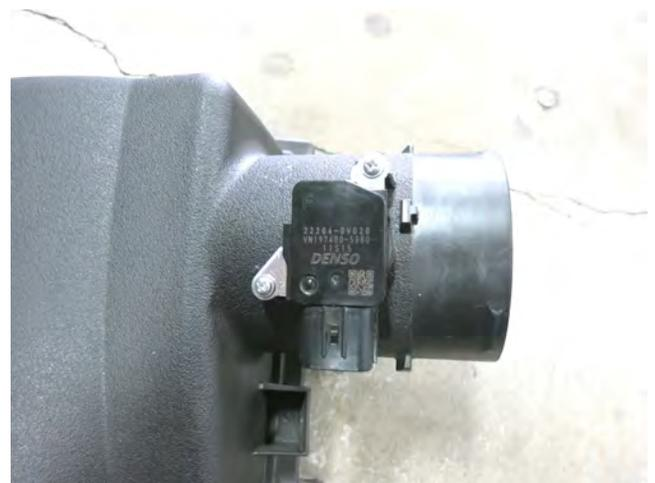
j. Use a small Phillips head screwdriver to unfasten the 2 Phillips head screws and remove the MAF sensor from the upper air box. Do not discard any of the stock equipment removed thus far.
