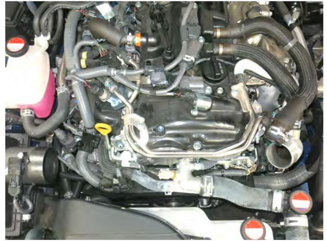
f. Loosen the hose clamp holding the intake tube onto the turbo inlet pipe. Then, remove the intake tube.
