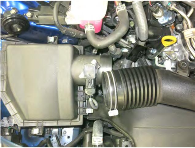
e. Use a 10mm socket and ratchet, or a Phillips head screwdriver, to loosen the hose clamp holding the intake tube to the air box. Then, pull the intake tube off of the air box.
