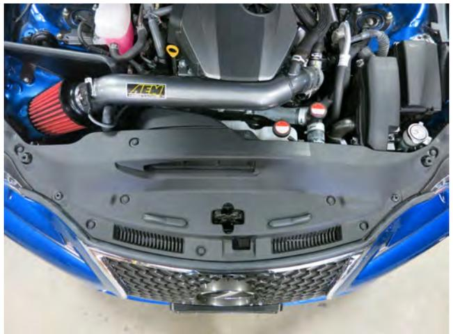
q. Replace the radiator shroud with the 9 push clips you removed in step 2a.
