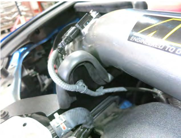
n. Clip the MAF harness onto the heat shield with the two wire ties. Then plug the harness back into the MAF sensor.
