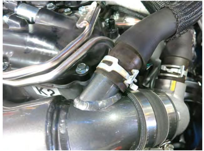
m. Reattach the breather hose to the port on the intake pipe.
