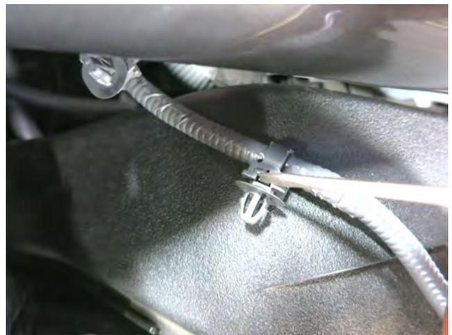
o. If there is too much tension on the MAF sensor harness, you can adjust the position of the wire ties. Use a small flat head screwdriver to relieve tension on the wire tie. Then, you can slide the wire tie along the harness as necessary.
