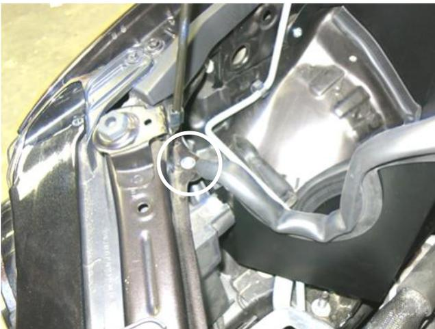
e. Make sure the AEM heat shield is under the lip of the core support, and install the provided bolt/nylon washer securing the AEM heat shield to the vehicle. **NOTE: On vehicles equipped with projector head lights it will be necessary to install the bolt from the bottom up.**
