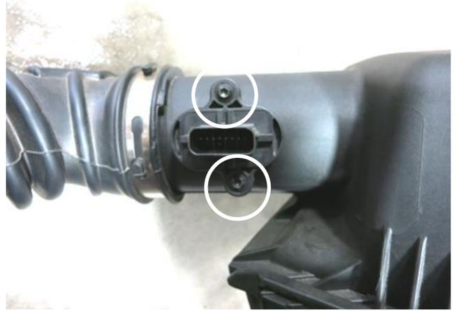
f. Remove the two screws securing the mass air sensor to the stock upper air box. The screws will not be re-used, however the mass air sensor will be reused in step 3g.
