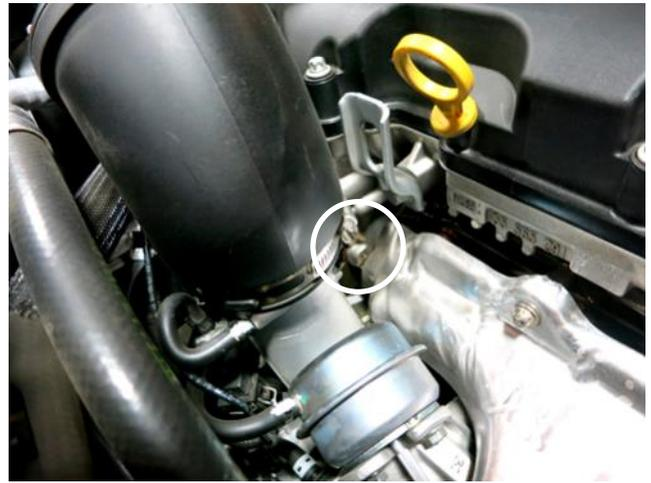
b. Loosen the hose clamp at the turbo compressor inlet.
