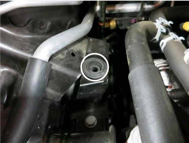
a. Take the rubber grommet that was removed in step 2e. and install it into the same location the rubber grommet in step 2d. was removed.
