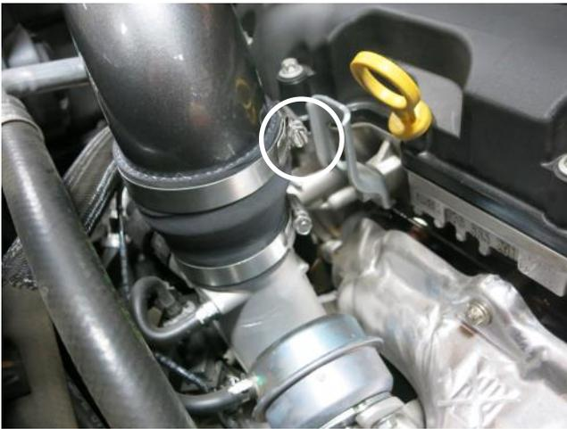
i. Install the AEM intake tube into the vehicle aligning the tube with the coupler. Tighten the hose clamp (circled above) at this time.
