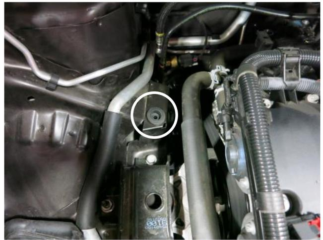
d. Remove the rubber grommet from the vehicle. This will not be reused.
