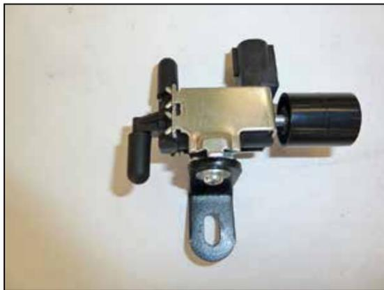
13. Install the provided vacuum caps and "L" bracket onto the vacuum solenoid using the provided hardware.
