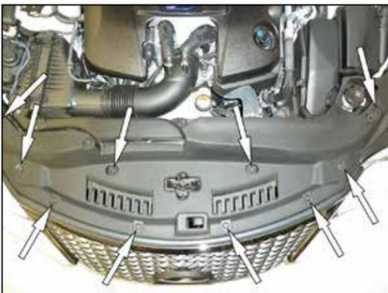
6. Remove the ten push pins that secure the core support shroud and then remove the core support shroud from the vehicle.
