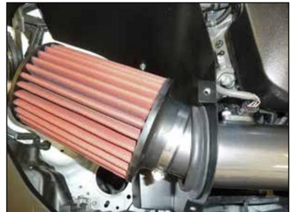
18. Install the AEM® air filter onto the intake tube and secure with the provided hose clamp.
