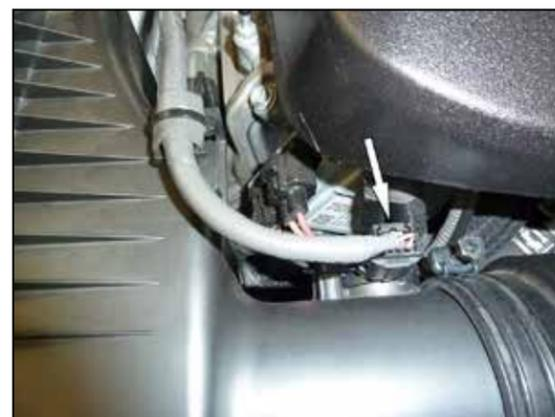
3. Disconnect the mass air sensor electrical connection and unhook the wiring harness.
