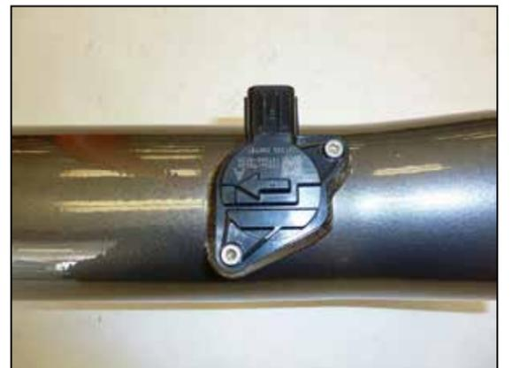
16. Remove the mass air sensor from the factory air filter housing and install it into the AEM® intake tube.
