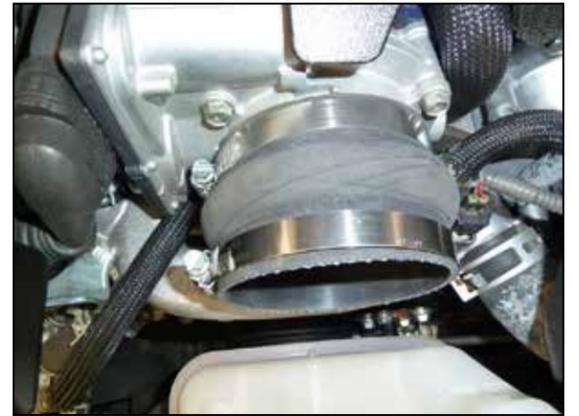
15. Install the provided hump coupler onto the throttle body and secure with the provided hose clamp.
