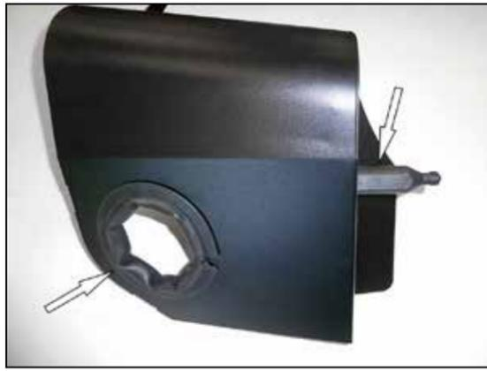
9. Install the 13.5" section of edge trim into the hole of the heat shield. Install the heat shield mounting post onto the heat shield using the provided hardware.
