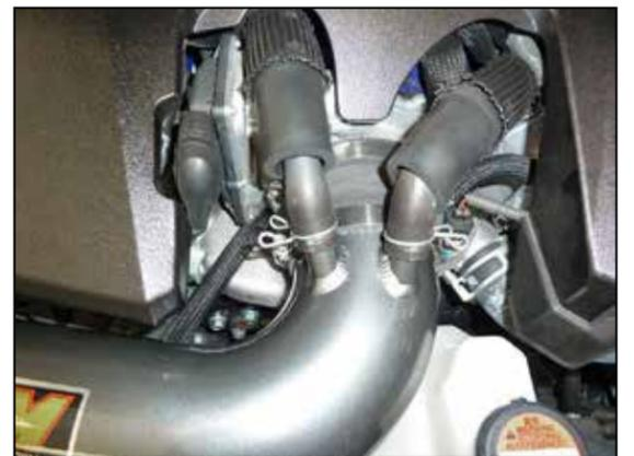
17. Install the AEM® intake tube through the heat shield and into the coupler on the throttle body. Adjust the tube for best fit and then secure with the provided hose clamp. Connect the crank case vent lines and secure with the factory spring clamps.
