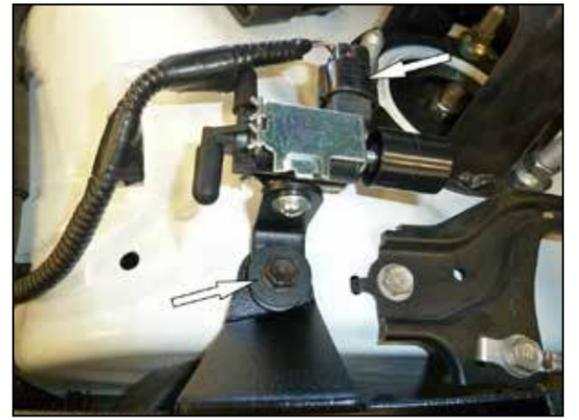
14. Using the factory bolt from step 4, secure the vacuum switching valve and heat shield to the shock tower as shown.
