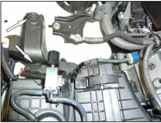
4. Disconnect the vacuum switching valve electrical connection. Remove the bolt which secures the air filter housing to the strut tower.
