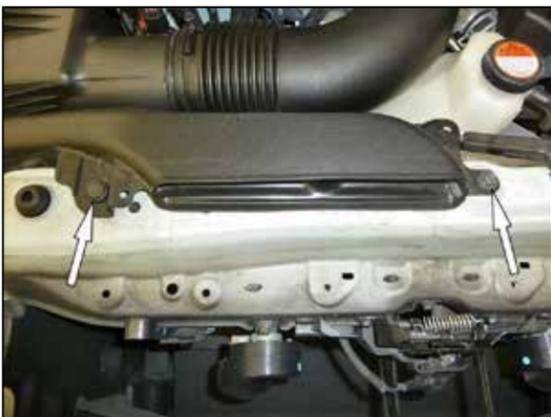
7. Remove the bolt and push pin that secure fresh air intake duct, then remove the fresh air duct and air filter housing from the vehicle.
