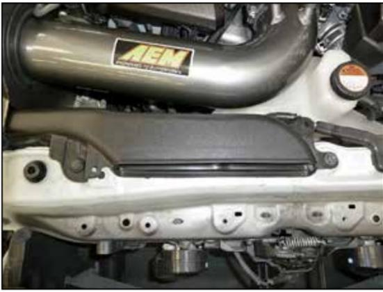
19. Reinstall the fresh air intake duct and secure with the factory Hardware.
