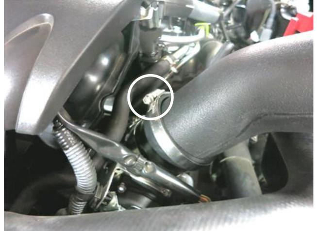
h. Insert the upper intake tube (9-6791) into the throttle body coupler. Use the supplied hose clamp to loosely secure in place.
