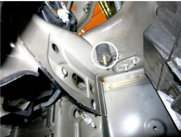
c. Install the rubber mount in the indicated hole, secure with a provided washer and nut.
