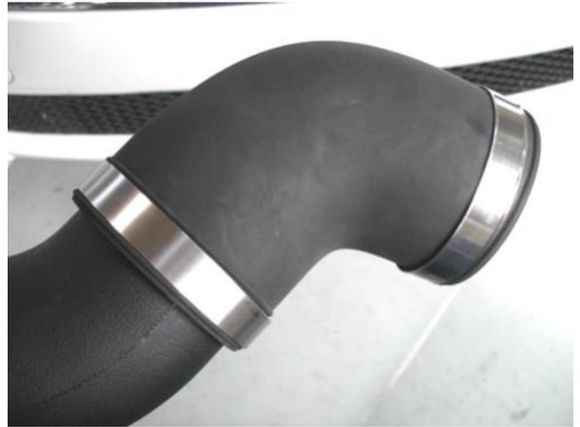
f. Attach the 90° elbow coupler onto the upper intake tube (side opposite of the nipple). Slide the supplied hose clamps onto each end of the coupler.
