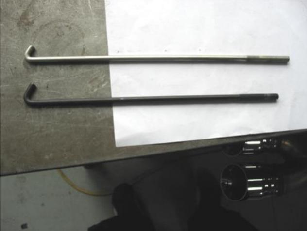
a. Replace the factory j-hook with the shorter j-hook and tighten the with the nut that was removed in step 2i.
