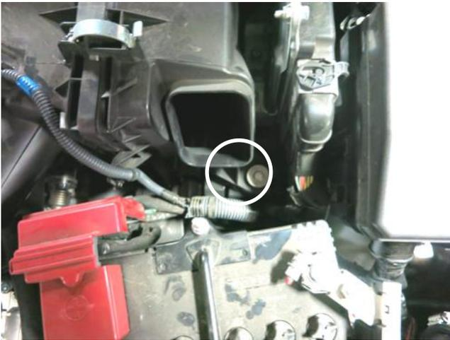
g. Remove the bolt that holds the factory air box in the engine compartment.
