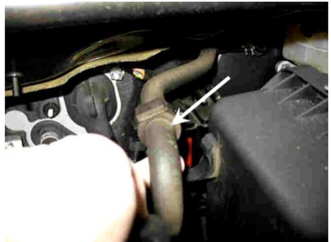
d. Unclip the hose from the air box retainer.
