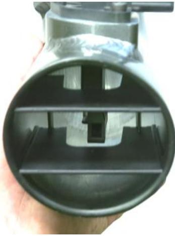
e. Install the supplied MAF insert into the AEM intake tube as shown. Note: Apply a few drops of super glue to the lip of the MAF insert to secure it in position.
