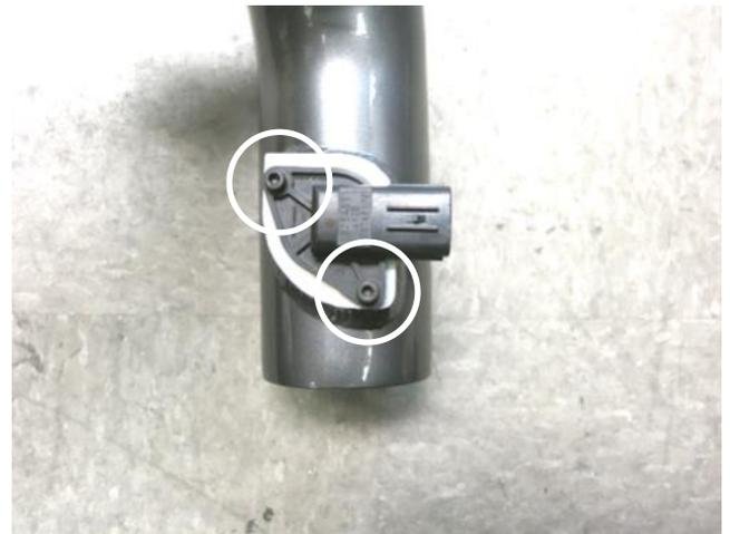
d. Install the MAF that was removed in step 2m. into the AEM intake tube and secure with the supplied hardware.
