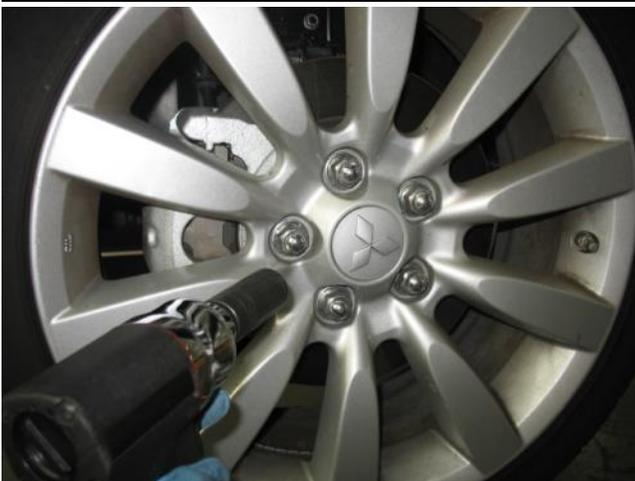
o. Re-install the wheel that was removed in step 2k. onto the vehicle and torque the lug nuts to the manufacturer's torque specifications.
