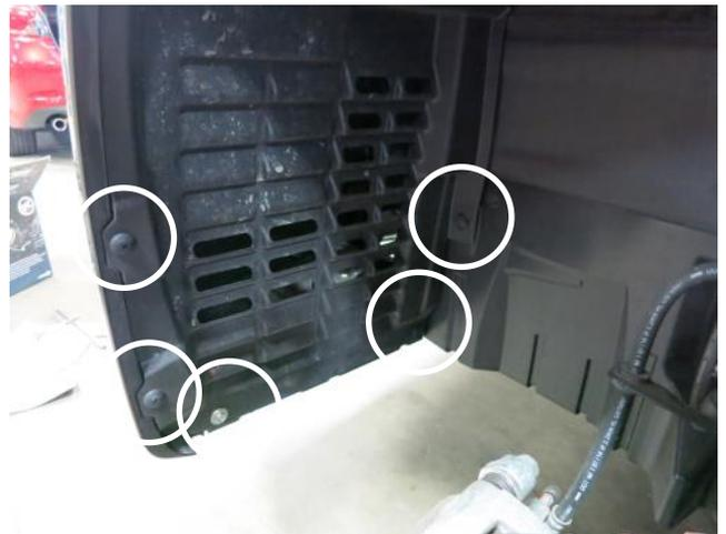
n. Re-install the wheel well liner with the existing hardware that was removed in step 2l.
