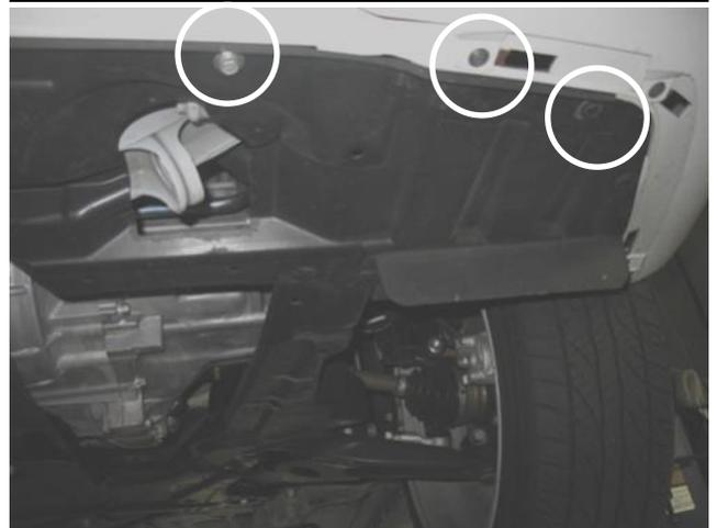
p. Re-install the plastic trim with hardware that was removed in step 2j. Remove the jack stands and lower the vehicle back onto the ground.
