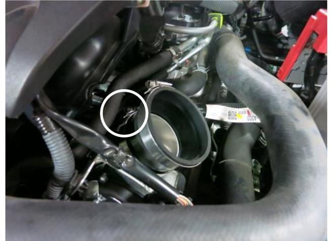
b. Install the supplied coupler and hose clamps onto the throttle body. Tighten the hose clamp circled at this time.
