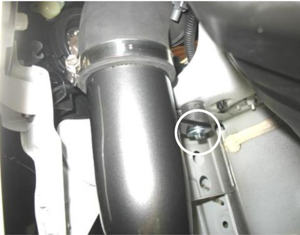
k. Route the lower intake tube through the bottom of the fender well. Align the intake tube's bracket onto the rubber mount and secure in place with the supplied washer and nut. Tighten the hose clamp on the coupler.
