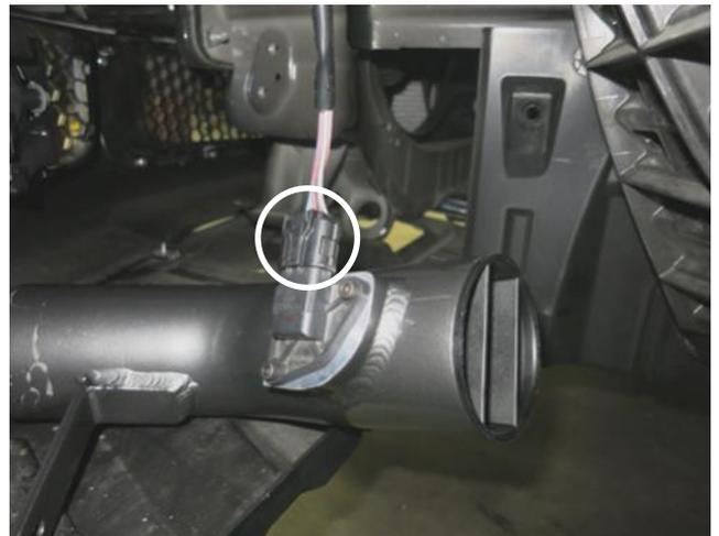
j. Plug the MAF extension harness into the MAF sensor.
