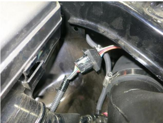
i. Connect the extension harness to the factory connector and route the MAF sensor harness down into the wheel well area.
