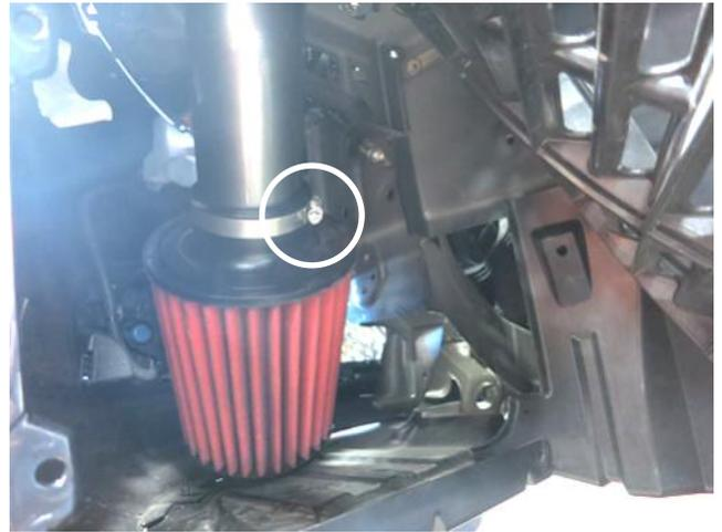
l. Install the AEM air filter onto the lower end of the intake tube and secure with the supplied hose clamp (9444). Once both tubes and filter are properly aligned go back and tighten all the hose clamps throughout the intake system.
