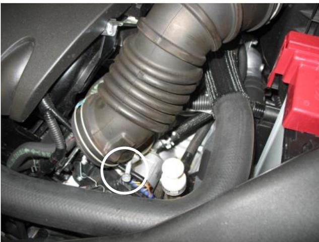
c. Loosen the hose clamp on the intake hose at the throttle body.
