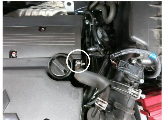
b. Release the spring clamp and remove the PCV hose from the crankcase side.
