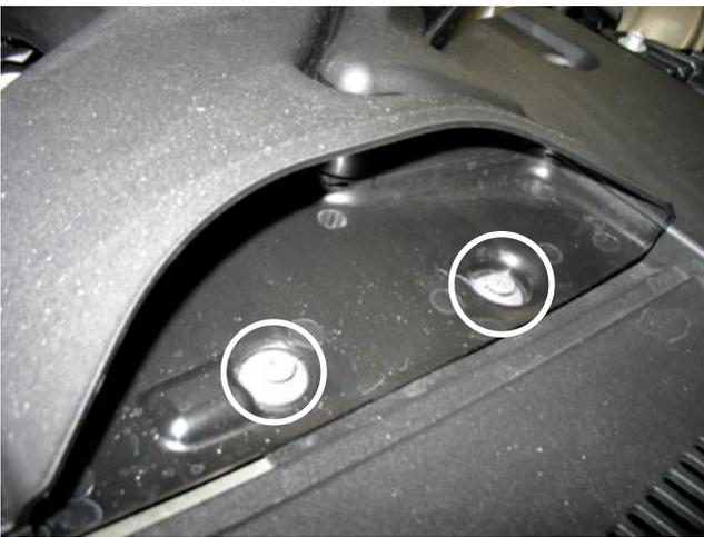
a. Remove the two Phillips fasteners that secure the fresh air duct to the core support and remove the fresh air duct from the engine compartment.
