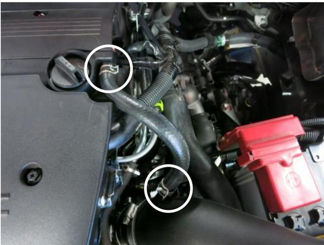
m. Attach the supplied PCV hose onto the crankcase inlet and intake pipe nipple. Secure each end with the spring factory clamps removed in step 2n.
