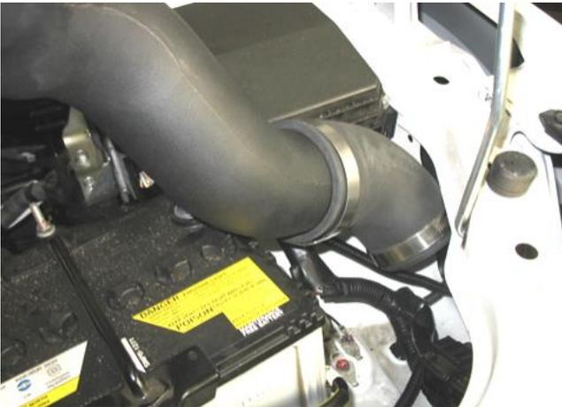
g. Route the intake tube down through the wheel well opening as shown.
