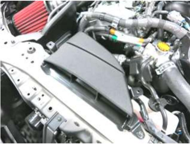
k. Reinstall the stock air duct into the heat shield and fasten down using the original bolt from step 2c.
