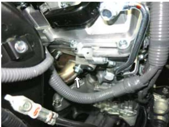
c. Loosely install the provided M8 bolt(1-2066) and washer(559960) into the threaded hole located on the engine block.
