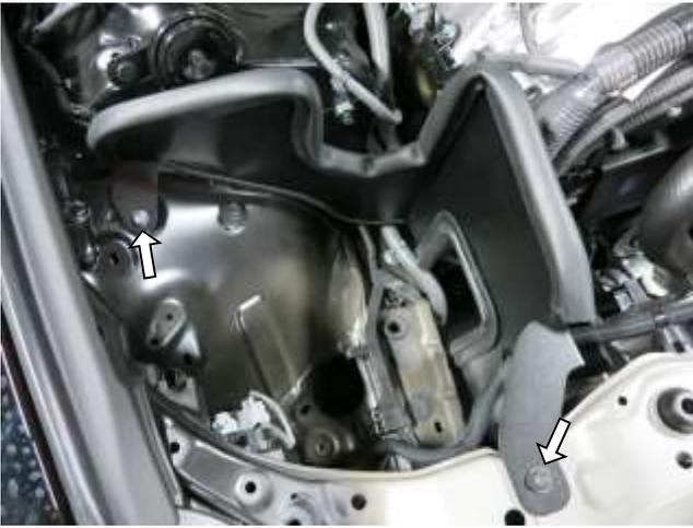
e. Install the AEM heat shield as shown and fasten the inner tab with the m6 bolt(1-2038). Fasten the upper tab using the bolt removed in step 3b.
