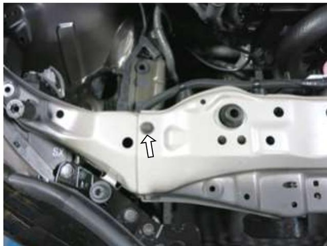
b. Remove the indicated bolt using a 10mm socket. Set this bolt aside for use with the AEM heat shield installation.
