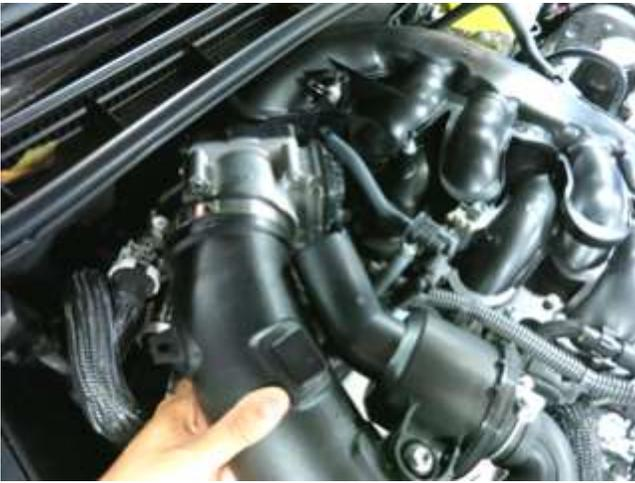
g. Loosen the hose clamp and slide the stock tube off the throttle. Remove the stock intake system.
