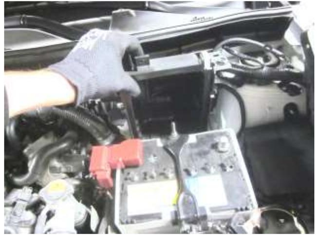
f. Remove the stock air box from the vehicle. **Note:** Remove the rubber bushings under the air box and keep with air box as they will not be utilized.
