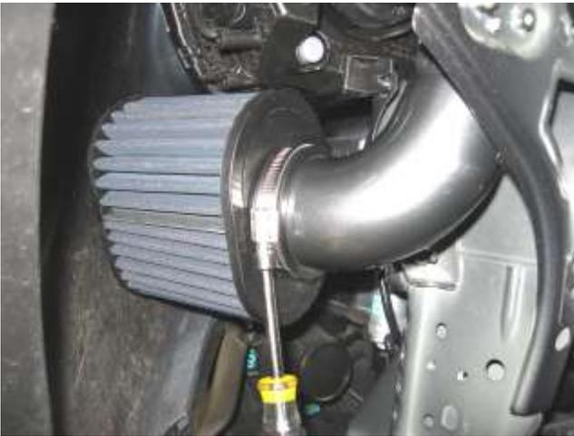
g. Install the AEM air filter onto the intake tube and tighten the provided hose clamp. On some trim models, the air filter may need to be rotated to fit properly.
