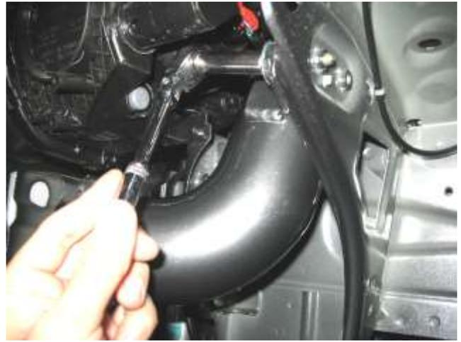
f. Align the lower portion of the AEM intake tube bracket on top of the rubber bushing and tighten the provided M6 nut/washer.
