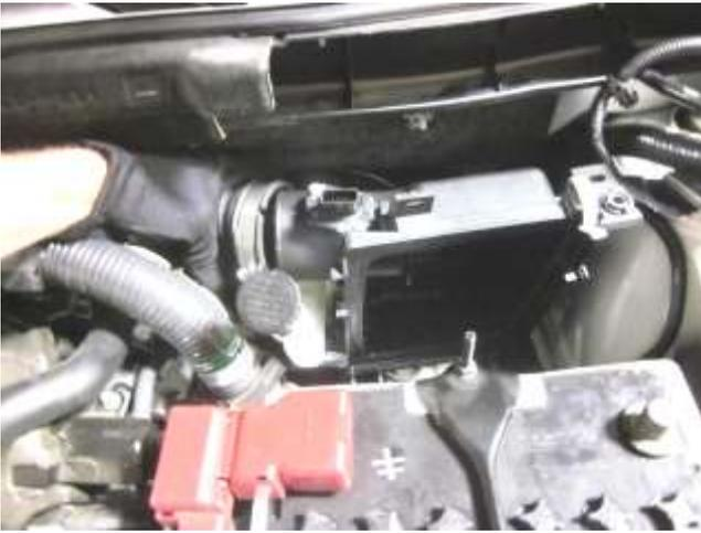
e. Disconnect the stock intake tube from the air box.
