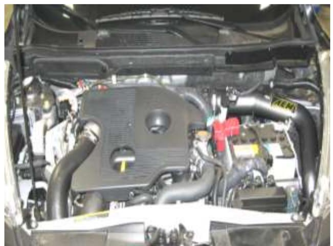
j. Finished installation of AEM Intake System.
