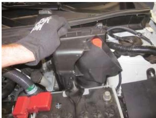
d. Remove the upper half of the air box with the filter still intact and lift both out of the engine compartment.
