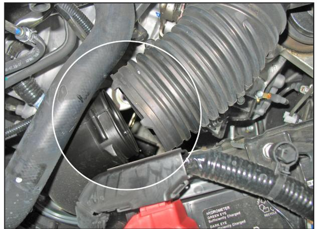
h. Disconnect the lower rubber inlet tube connecting the lower air box to the plastic inlet tube routed through the bottom of the vehicle.
