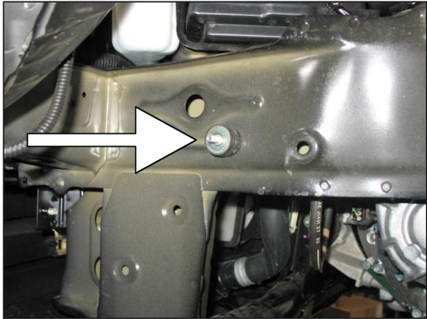
k. Screw the rubber mount into the threaded hole of vehicle's frame.
