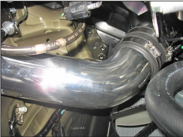
l. Route the lower intake pipe into the engine bay and attach the upper end to the upper intakes pipe's coupler.
