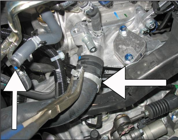
j. **NOTE: Ensure the engine is completely cool before removing the coolant hose, or hot coolant will escape from the cooling system and cause injury or damage. To do this, the radiator coolant must first be drained. Follow the procedure described in your vehicle's factory service manual to drain the coolant. Be sure to capture the coolant in a clean container so it can be recycled back into the system in a later step.**
