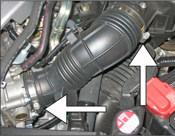
e. Loosen the two hose clamps securing the rubber inlet tube to the stock air box and the throttle body. Remove the rubber inlet tube from the vehicle.
