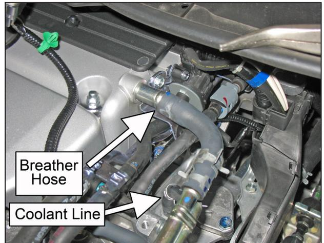
m. Disconnect the breather hose from the valve cover and disconnect the small coolant line connecting the engine to the hard lines.
