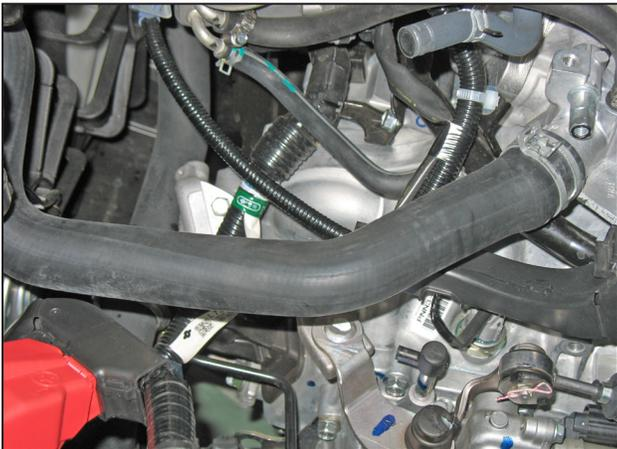
f. Route the radiator hose as shown. Trim the battery tray for clearance if necessary.
