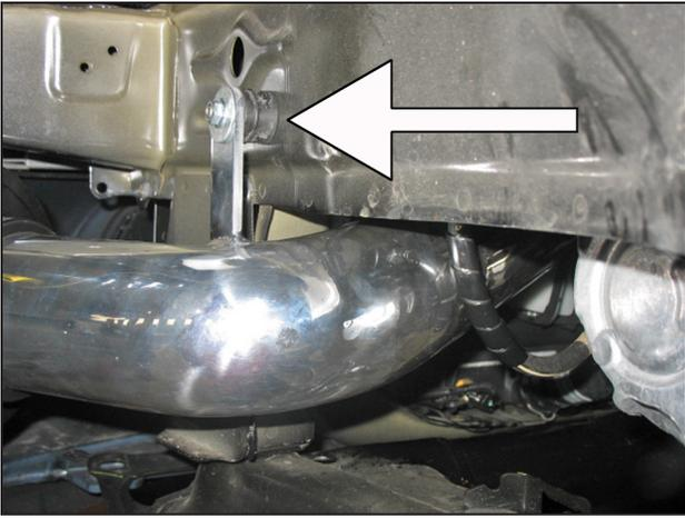
n. Loosely secure the lower intake pipe's bracket to the rubber mount installed in step 3k. Secure the bracket with the supplied washer and serrated nut.
