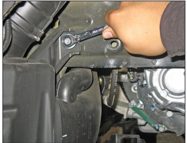
q. Remove the bolt securing the resonator to the inner fender well.
