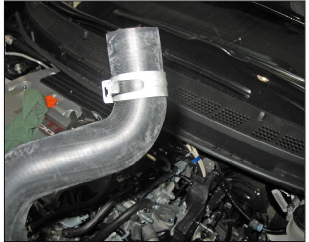
e. Install the supplied radiator hose using the stock hose clamps.
