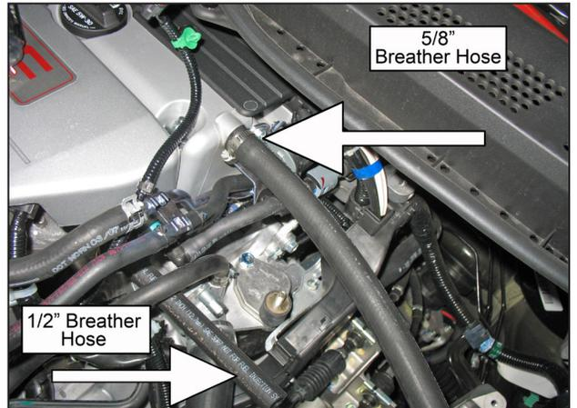
g. Install the two supplied breather hoses, one to the valve cover and the other to the small plastic valve located on the engine. Secure each hose with the supplied hose clamps.
