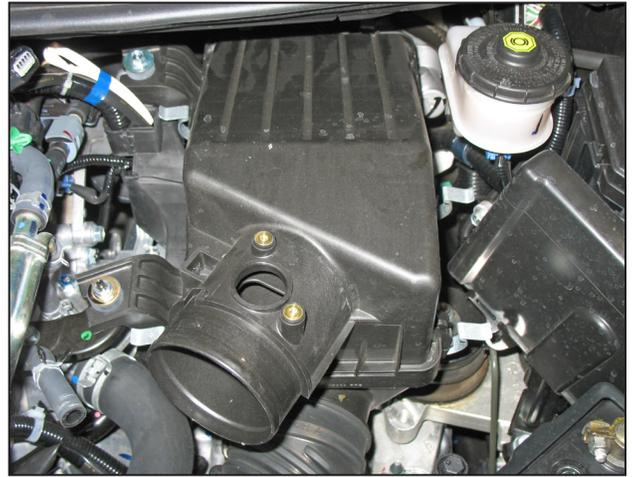
f. Remove the MAF sensor from the air box. Unclip the upper air box from the lower air box.
