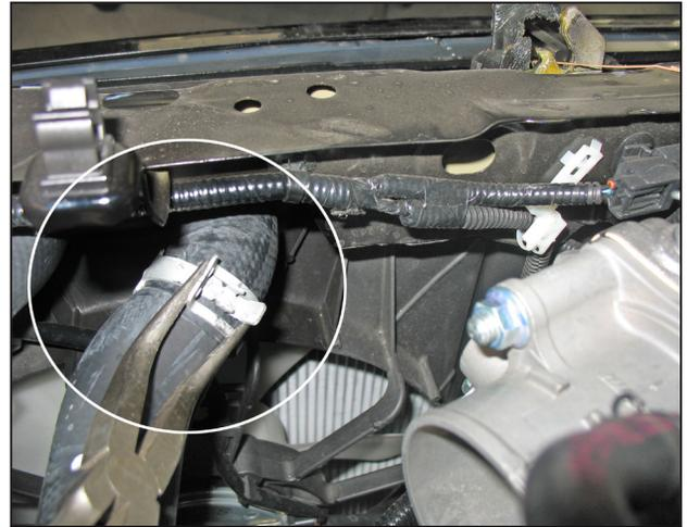
k. Using pliers remove the clamp securing the upper radiator hose to radiator. Remove the upper radiator hose from the vehicle.
