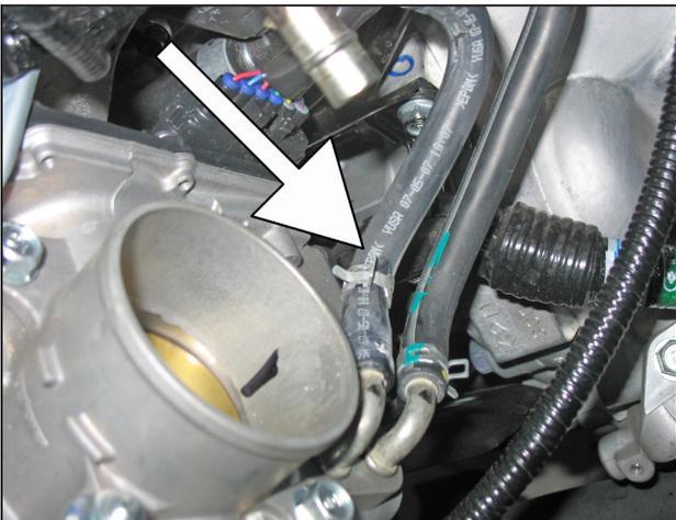
l. Disconnect the coolant line connected to the throttle body.
