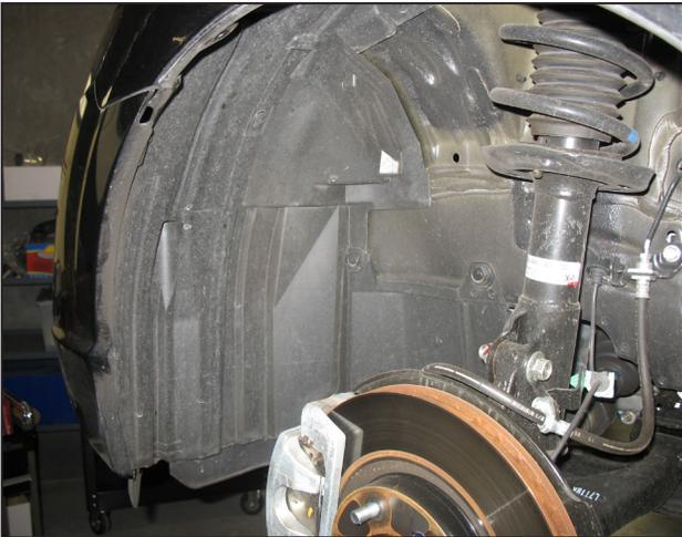
p. Remove the fender liner on the driver side wheel.
