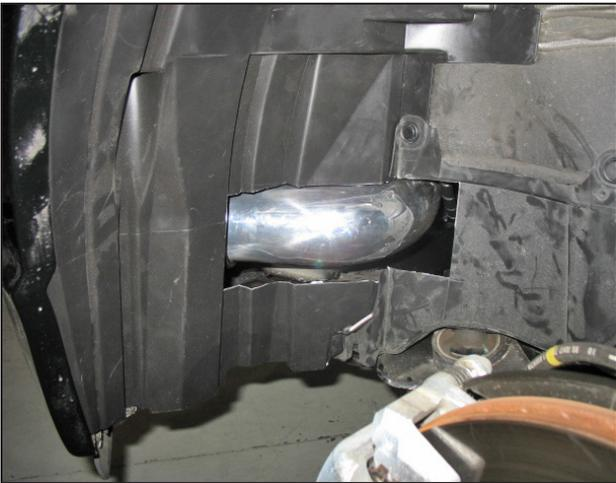
p. Install the fender liner and any hardware that was removed in step 2p. Trim the fender liner to allow clearance for the lower intake pipe.
