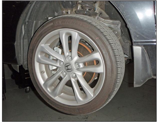
o. Raise the front of the vehicle with a jack. Refer to your owner's manual for proper jack and jack stand placement to properly support vehicle. Support your vehicle using properly rated jack stands before wheel removal or while working under the vehicle. **NEVER WORK UNDER A VEHICLE WITHOUT USING JACK STANDS.** Remove the driver side wheel.
