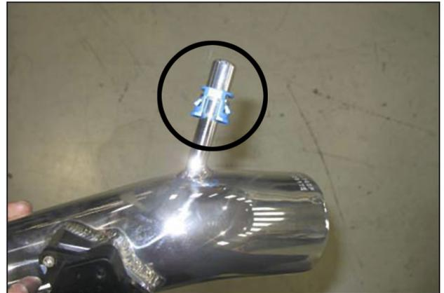
c. Install the plastic breather hose clip (removed in step 2l) onto the nipple of the upper intake pipe. Simply slide the clip over the end until it snaps into place.
