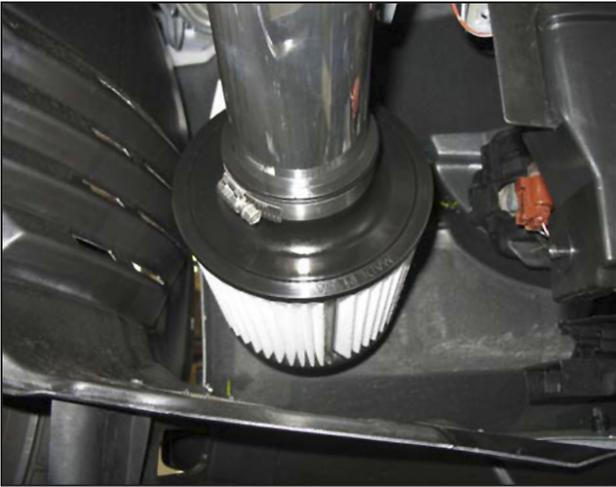
l. Install the air filter onto the end of the lower intake pipe. Push the air filter over the intake pipe until the stop in the air filter is reached. Secure the air filter onto the intake pipe with a #48 hose clamp.
