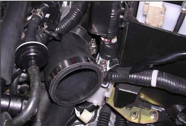
b. Install the 45-degree coupler onto the turbo inlet and secure using a #40 hose clamp.
