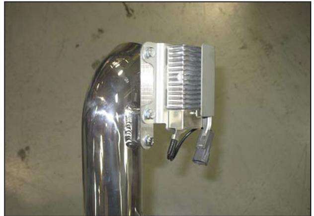
i. Attach the resistor ballast to the lower intake pipe using the mounting bracket, three M6 bolts, three washers, and one M6 nut.
