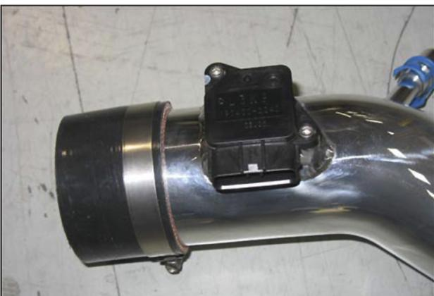
d. Install the MAF sensor into the upper intake pipe with the provided 8-32 bolts. Install the 2.75" straight coupler onto the intake pipe end closest to the MAF sensor.
