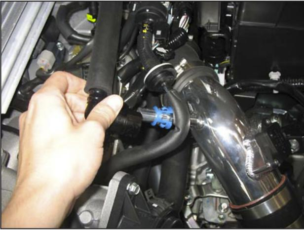
f. Install the upper intake pipe into the 45-degree coupler on the turbo inlet. Rotate the intake pipe until the breather hose aligns with the intake pipe's nipple. Attach the breather hose to the intake pipe nipple and connect the MAF sensor harness connector to the MAF sensor.
