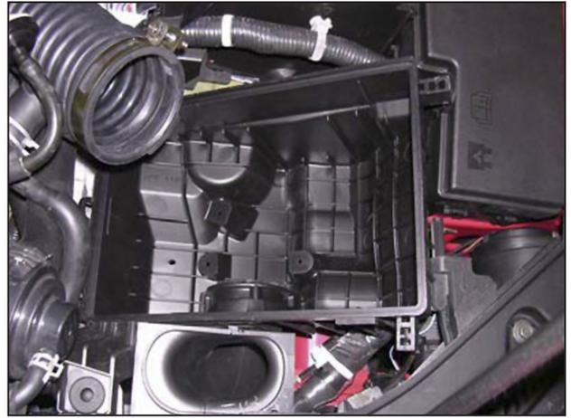
f. Remove the check tab on the backside of the air filter housing, then slide the rubber isolator rearward. Lift up on the lower air filter housing and remove.
