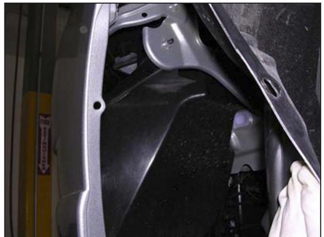
j. Remove the three bolts and the two plastic screw connectors securing the inner fender liner. Position the fender liner out of the way so the inner bumper/fender area can be accessed.
