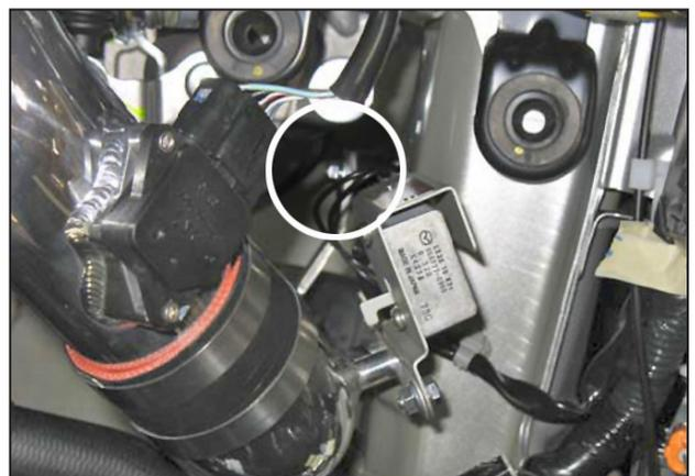
k. Secure the lower intake pipe's mounting bracket to the rubber mount with a M6 washer and nut. Reconnect the wiring harness to the resistor ballast.
