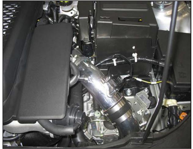
m. Reinstall the intercooler cover and check for clearance. Adjust the intake pipes if necessary.
