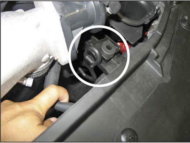
e. Remove the air filter from the housing. Remove the rubber strap securing the front of the lower housing by pulling up on the loop.
