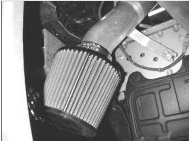
l. Install the AEM® air filter onto the end of the lower intake pipe. Make sure the air filter is fully and squarely seated on the end of the pipe. Use a #52 hose clamp to secure it in place.
