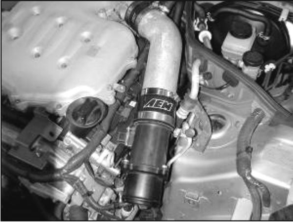
f. Install the assembly from step 3c on the upper intake pipe. Loosely install a #48 hose clamp on the coupler. Make sure the MAF sensor connector is pointing toward the oil cap.
