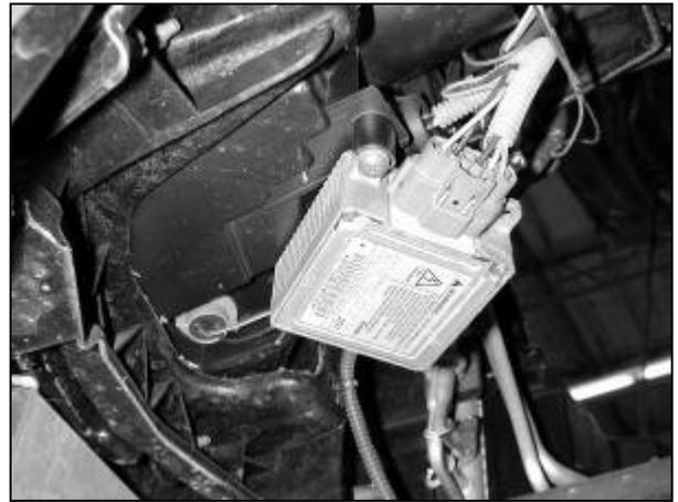
i. If installing on a G35 Sedan, remove the mounting screw for the HID headlight controller.
