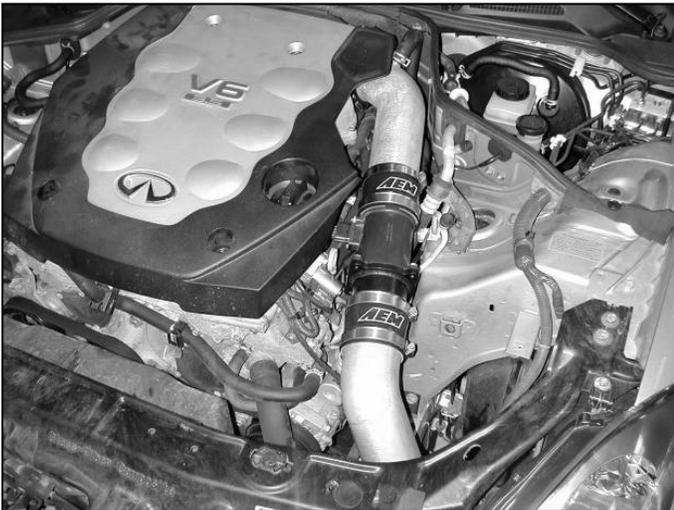
n. Check closely for clearance around the air filter and the AEM® MAF sensor adaptor, reposition as needed.
