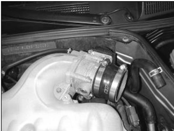
d. Place the 3.25"-3.0" reducing silicone coupler on the throttle body. Use a #52 hose clamp around the throttle body. Make sure the coupler is sitting squarely on the throttle body and tighten the #52 hose clamp. Loosely install a #48 hose clamp on the other end of the coupler.
