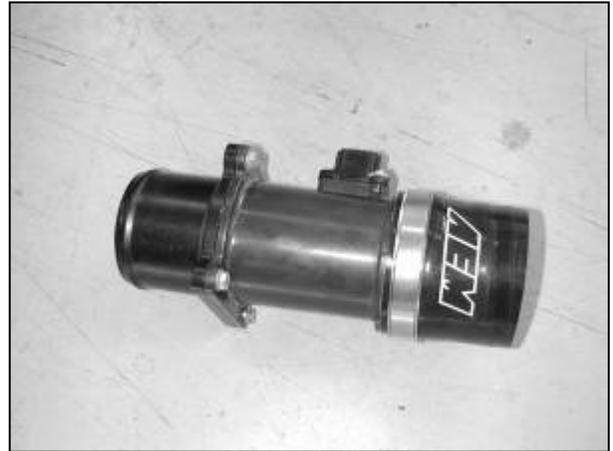
c. Slide one of the 3" straight silicone couplers over the MAF sensor as shown. Lightly oiling the inside of the coupler may help. Secure the coupler in place using a #48 hose clamp.
