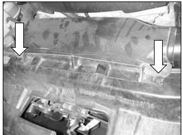
b. Remove the two plastic fasteners holding on the air duct and remove the duct from the engine bay.
