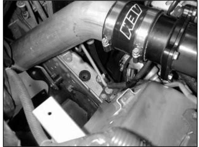
k. Install the lower intake pipe in the end of the coupler on the AEM® MAF adaptor. Line up the bracket on the pipe with the rubber mount and install the 6mm nylock nut and fender washer (See diagram below). Do not completely tighten.
