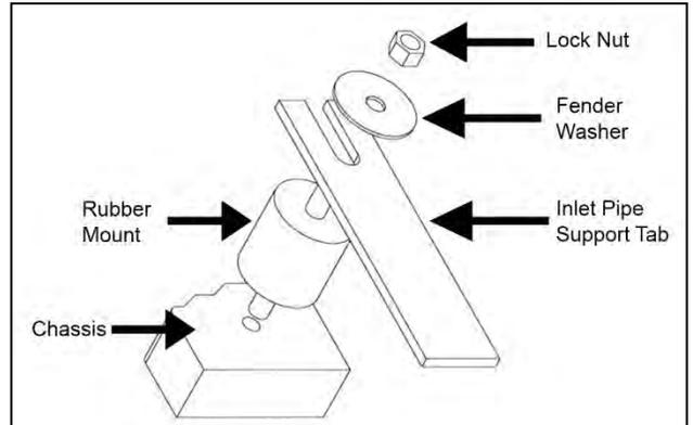
Proper installation of rubber mount assembly.
