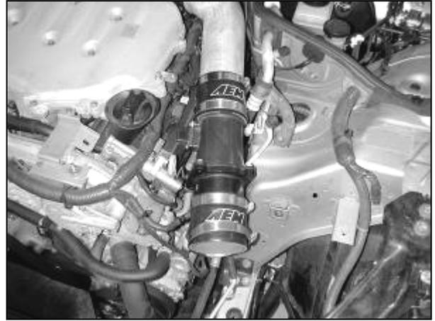
g. Install the other 3" silicone coupler on the end of the AEM® MAF adaptor. Loosely install two #48 hose clamps.
