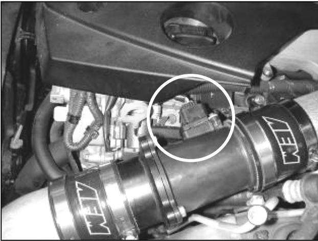
m. Plug in the MAF sensor. Place the engine cover on the intake manifold and check for clearance of the MAF sensor plug. Rotate the MAF sensor assembly until the plug has adequate clearance of the cover.
