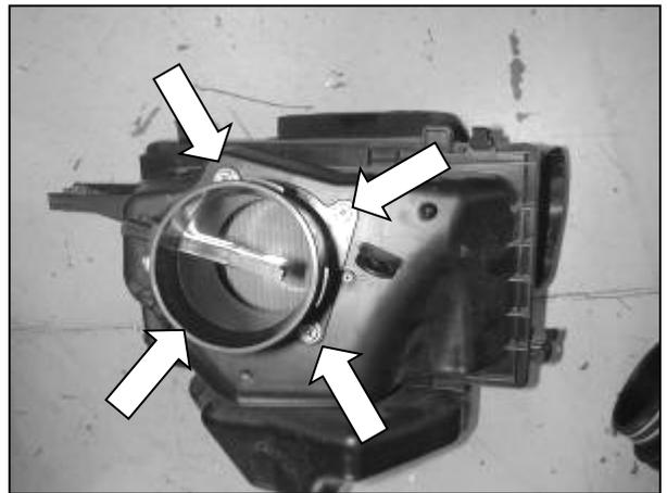
j. Remove the four bolts holding the MAF sensor on the factory air box. Handle the MAF sensor with care.
