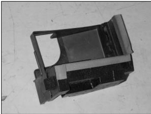
**NOTE:** The G35 sedan has foam insert attached to the plastic duct. Remove the whole assembly.
