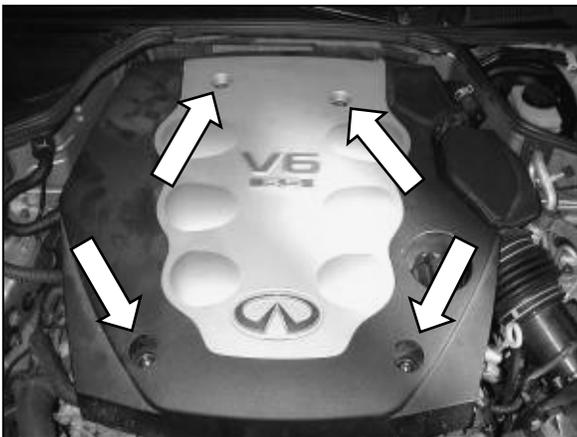
a. Remove the four fasteners holding on the engine cover. Remove the engine cover.
