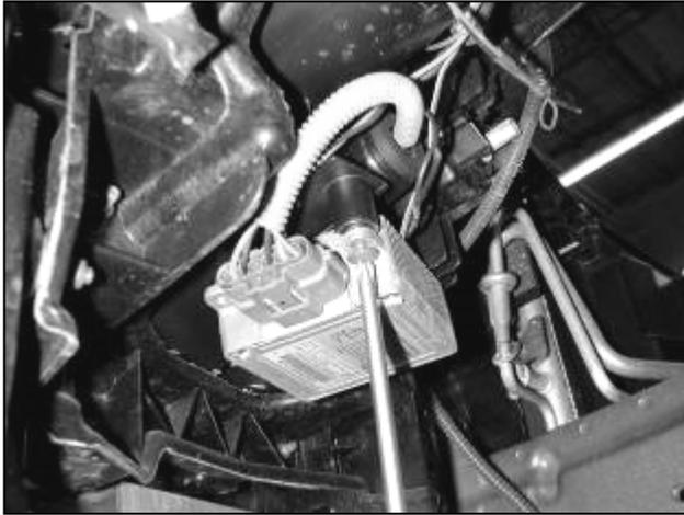
j. Rotate the HID controller forward and reinstall the screw in the other mounting hole on the controller. Pull excess slack for the wires from farther up the harness if needed.
