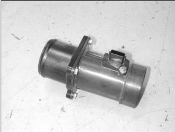
b. Using the 6mm bolts and washers included in the kit, bolt the MAF sensor to the AEM® adaptor.
