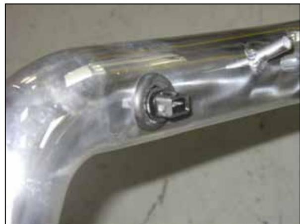
e. Install the supplied grommet into the hole on the inlet pipe. Gently press the IAT sensor into the grommet as shown.
