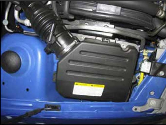
e. Loosen and remove the three bolts securing the air filter housing to the chassis. Remove the housing and the inlet hose by lifting straight up.
