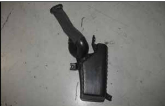
i. Remove the lower intake resonator.
