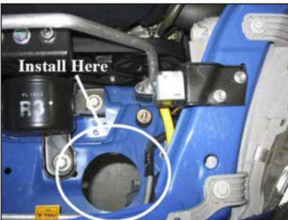
d. Install the supplied rubber edge trim around the hole in the inner fender.
