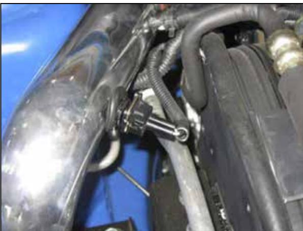
j. Plug the wiring harness into the IAT sensor mounted in the intake pipe. Route the wires under the inlet pipe to avoid scratching the pipe's finish.
