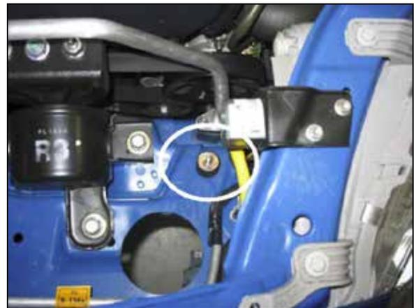
c. Locate the front threaded hole where the stock air filter housing was secured. Thread the supplied rubber mount into the hole in the engine compartment as shown.
