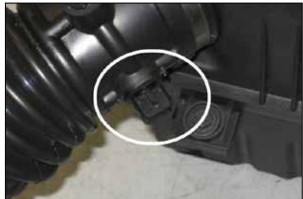
j. Remove the inlet air temperature (IAT) sensor from the stock inlet tube. This may be glued in place so use a sharp knife to cut the glue along the gap and pull the IAT out of the tube.
