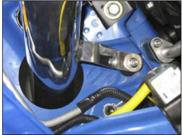
g. Align the inlet pipe mounting bracket with the previously installed rubber mount. Secure the bracket using the supplied M6 washer and nut.
