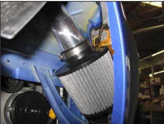
h. Install the air filter on to the end of the lower inlet pipe. Push the filter over the pipe until the stop in the filter is reached. Use a #44 clamp to secure the filter onto the inlet pipe.
