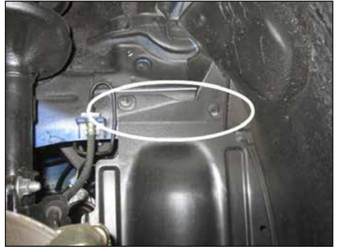
f. From the passenger side wheel well, remove the nut and bolt securing the inner splash shield to the chassis.
