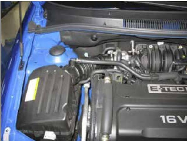
a. Stock air box system installed.
