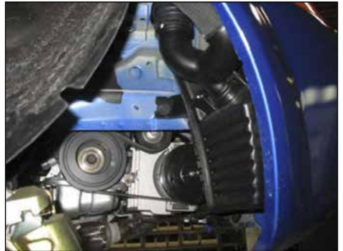
h. Remove the two bolts, one plastic nut, and the plastic retaining clip on the lower resonator and resonator inlet pipe respectively.
