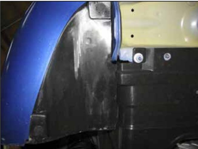
g. From underneath the vehicle remove the two bolts and two plastic connectors holding the splash shields in place. Remove the lower shield and move the fender well liner out of the way.
