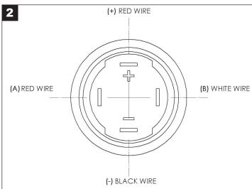
WITH THE SWITCH IN PLACE, PLUG THE 4-WIRE CONNECTOR HOUSING INTO THE BACK OF THE SWITCH TERMINALS FOLLOWING THE DIAGRAM ABOVE. WE RECOMMEND RUNNING THE DOME LIGHT TO A SWITCHED OR IGNITION SOURCE AS THE AMBER HALO IS ALWAYS ON. THE AMBER HALO HAS A DRAW OF 15 MILLIAMPS.
