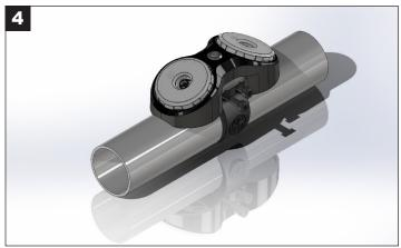
TAKE YOUR ASSEMBLED DOME LIGHT HOUSING AND CLAWS, HOLD IT INTO THE POSITION OF YOUR DESIRED LOCATION. TIGHTEN DOWN THE BOLTS WITH A 5MM HEX BIT. ROUTE THE WIRING TO NOT GET PINCHED ANYWHERE. THE MAIN SOURCE SHOULD BE FUSED AT 5 AMPS.
