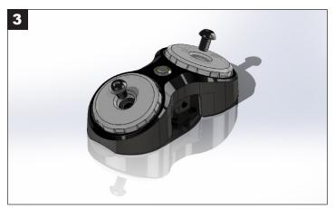
INSTALL YOUR TWO CYCLONES INTO THE MOUNT AND ROUTE THE WIRES THROUGH THE ACCESS HOLES. BOLT THE CYCLONES DOWN INTO THE THREADED HOLES OF THE HOUSING. CONNECT THE BULLET CONNECTORS TO THE APPROPRIATE CONNECTORS ON THE HARNESS. WE RECOMMEND WHITE DIFFUSED CYCLONES FOR INTERIOR SCENE LIGHTING.
