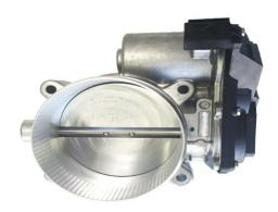
JET Throttle Bodies have preinstalled updated electronics. JET's CNC Machined 356 Aluminum Castings allows for increased air flow. This will allow for improved throttle response and more horsepower thru the entire driving range.
