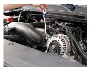
2. Loosen the clamp securing air intake tube to the throttle body.
