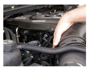
4. Disconnect breather tube from intake by gently pulling outwards. Loosen clamp at mass air sensor then remove intake tube.
