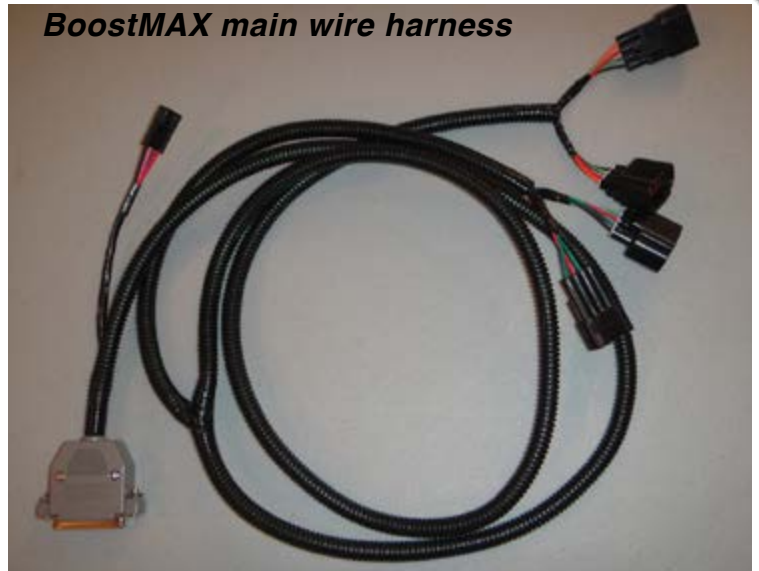
BoostMAX plugs into the Grey 25 pin connector
