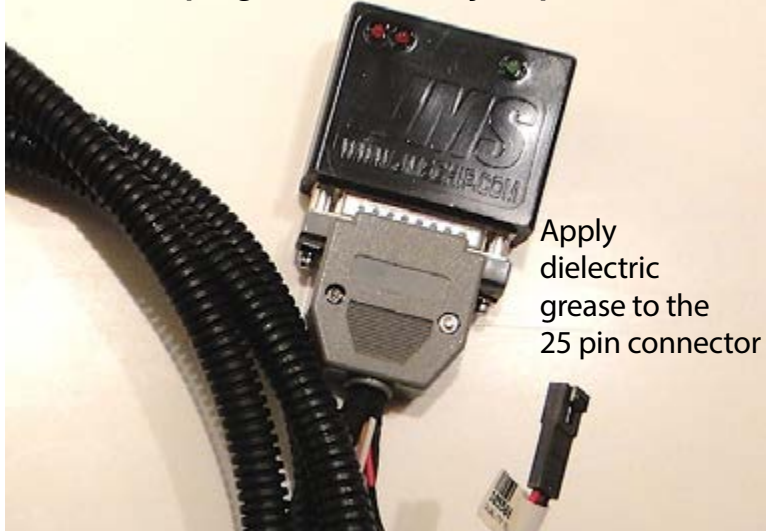
BoostMAX plugs into the Grey 25 pin connector
