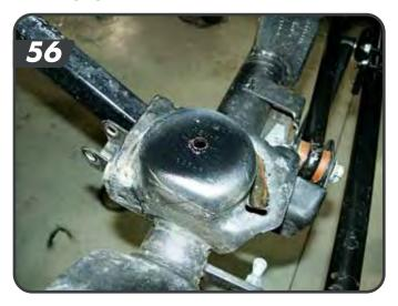
d. Place the provided bump stop extension inside one of the JSPEC front coil springs. Note: Taller springs are for the front. Install the front coil springs with the bump stop extension. Make sure the spring is seated properly in the axle mount.
