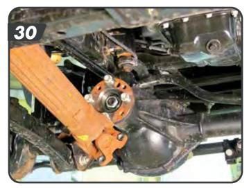
h. Disconnect the steering drag link from the pitman arm to ensure it doesn't bind when installing the new coil springs. Remove the tie rod end nut and dislodge the tie rod end from the pitman arm. Save nut. [31]
