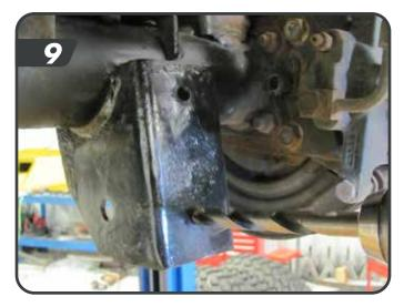
d. Place the JKS lower coilover mount over the factory bracket. Line the bracket up by temporarily installing the factory control arm bolt and line up the 2 rear holes. Use the provided 7/16" hardware to attach the bracket to the mount. The flange lock nuts can be placed on the bolts using a magnet from the top. Tighten hardware to to 70 ft lbs [11].
