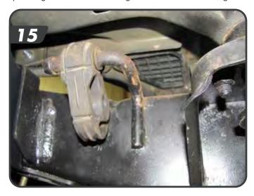
d. Measure in 1-5/8" from the frame rail and make a cut line across the factory shock mount to the crossmember. To avoid a lot of grinding, the crossmember side of the shock mount can be cut just past the weld as shown [16].
