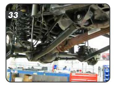
i. Mount the control arm to the frame rail bracket so the grease fitting is up on the flex eye. Install the original mounting bolt and nut. Finger tighten the bolt.
