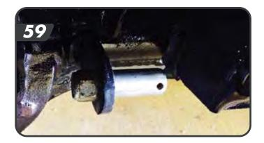
Note: In some cases a rotary grinder may be necessary to slightly open up the sway bar hole to clear the ½" bolt. This ensures a tight fit.
