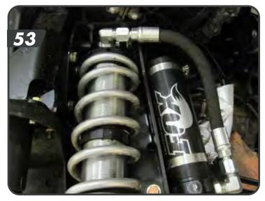
bk. Raise the axle to mount the coilover into the lower mount. Fasten with the  $\frac{1}{2}$ " x 2-34" bolt.
