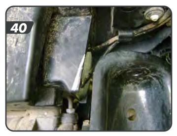
ai. The bottom of the plastic tray must be trimmed to provide clearance for the coilover bracket. Test the bracket fitment by temporarily holding up the main coil-over mount to the frame and lining up the OE brake line mounting hole to the lower hole in the bracket. Clearance as necessary. [41,42]
