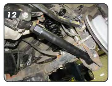
h. Mount the control arm to the frame bracket with the grease fitting up. Install the original mounting bolt and flag nut. Finger tighten the bolt. DO NOT torque mounting hardware until instructed.
