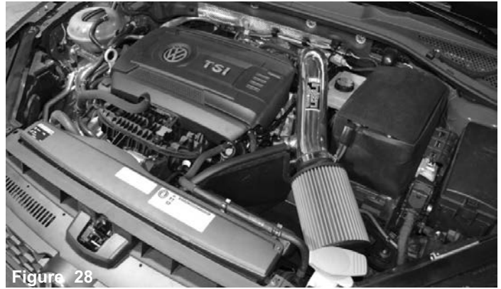
Congratulations! You have just completed the installation of this intake system. Periodically, check the alignment of the intake, normal wear and tear can cause nuts and bolts to come loose. Note: Check clearance and adjust if needed! Failure to check the alignment and adjust the intake can cause damage that will void the warranty. Injen Technology is not responsible for any damages caused by/from improper installation.
