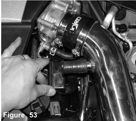
Figure 50 Once the pipe is aligned and there is clearance along the pipe, you may now tighten the clamp securing the pipe
