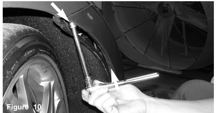
Figure 7 Passenger side strut tower- Loosen and remove two 14mm bolts and one 14mm flange nut from the stabilizer bar.
