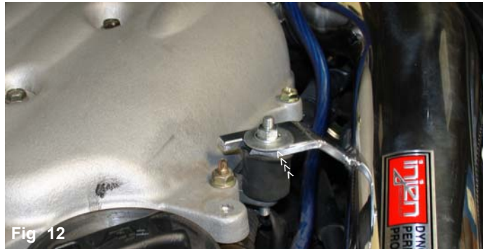
Fig 12 Once the intake is aligned use the m6 flange nut and fender washer to secure the intake in place.
