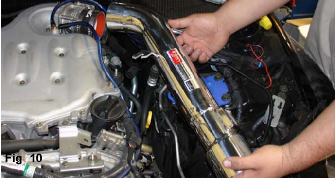
Fig 10 The crankcase breather line is attached to the intake port and the stock clamp is used to secure the line in place.
