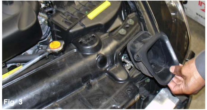
Fig 2 Loosen two nuts and remove the plastic intake manifold cover before installing the intake.
