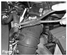
The tension clamp is compressed and pulled from the crank case vacuum hose located over the air intake duct.
