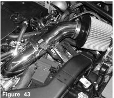
Check the entire intake system for best possible fit. Make sure there are no rubbing parts, rattles, or vacuum leaks, then continue to tighten all nuts, bolts and clips.
