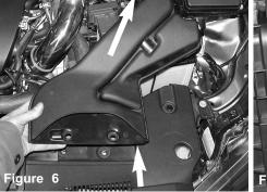
Pull up on the air scoop and pull forward in order to dislodge the air scoop from the air box cleaner.
