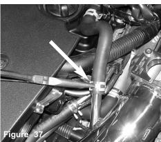
Use the needle nose pliers o compress the tension clamp to slip over the vacuum hose.
