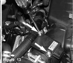
An allen screwdriver is used to loosen the two stock screws from the mass air flow sensor.
