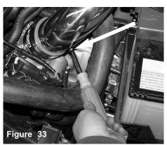
Once you have aligned the intake continue to tighten the hose clamp located over the intake, Page 4 of Part# SP1811
