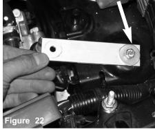
The extension bracket is placed over the pre-threaded hole that once held the air box cleaner in place. An m6 bolt and washer is used to fasten the bracket in place.
