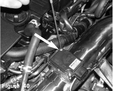
A an allen is used to fasten the screws over the mass air flow sensor.
