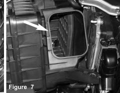
The air scoop is dislodged and pulled from the opening of the air box cleaner as shown above.
