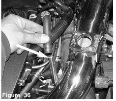
The crankcase vacuum hose is now pressed over the intake vacuum port.
