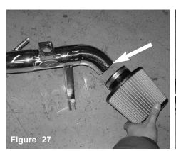
The filter is now aligned to the end of the intake.
