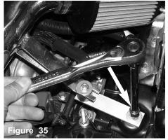
The m6 nut is now tightened over the extension bracket.
