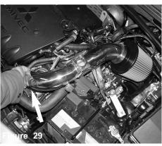
The assembled filter and intake is now lowered into the engine compartment.
