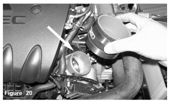
The 2 3/4" silicone elbow is pressed over the throttle body along with the clamps.
