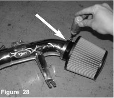
Once the filter has been properly adjusted, continue to tighten the filter clamp.
