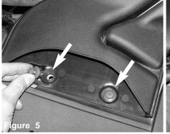
Once you have loosened the plastic clips, continue to pull up on the clips as shown above.
