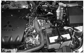
Shot of an empty engine compartment with no air intake box or air intake duct.
