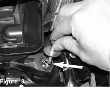
Once you have loosened the m6 bolt, continue to pull the m6 bolt out.
