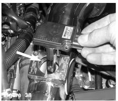
The mass air flow sensor is now inserted into the primary intake sensor adapter.
