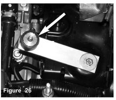
The vibra-mount is now installed as shown above.
