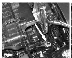
The m6 bolt is loosened from the base of the air box cleaner.
