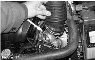
The air duct is now ready to be pulled off the throttle body.
