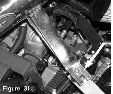
As the intake is inserted into the throttle body hose the intake bracket is aligned to the vibra-mount stud.
