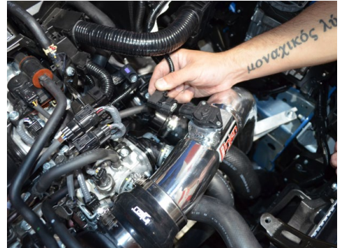
18. Reconnect the MAF sensor harness.
