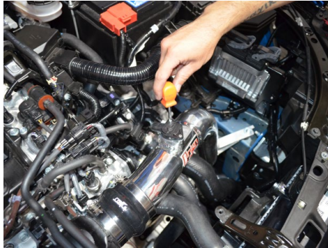
17. Install the MAF sensor onto the intake tube and secure using the OEM bolts.
