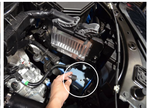
12. Mount the provided vibra mount to the the threaded hole on the chassis.
