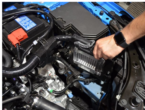
11. Remove the front bolt of the ECU bracket and then push the ECU towards the fuse box. This will make room for the vibra mount in figure 12.
