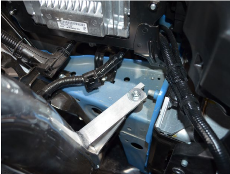
16. Secure the intake tube bracket with the provided M6 bolt and washer. Resecure the ECU to its factory position from figure 11.
