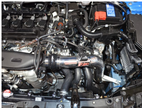
20. Adjust the intake tube for best fitment and then ensure all nuts, bolts, and clamps are properly secured.
