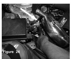
Position for best fit with filter clearance. There is a lot of movement for the intake tube position, re-tighten
