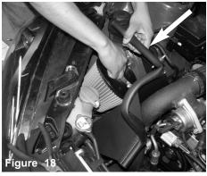
Install the heat shield into vehicle and position the tab to steps 11, place the filter inside of the heat shield prior to install.
