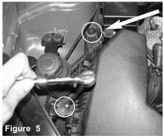
With 10mm socket and ratchet loosen the2 bolts holding in the stock air box.
