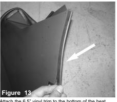
Attach the 6.5" vinyl trim to the bottom of the heat shield.
