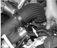
Position for easy clamp access, tighten clamp on intake tube using 8mm nut driver.
