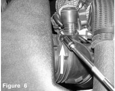
Loosen the clamp on the air box using 10mm socket and ratchet.
