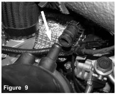
Remove the crank case line and brake booster line from the intake tube. Remove the diverter valve line from intake tube also.
