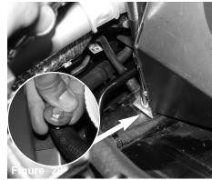
Install the provided hex screw with fender washer to the tab. Locate the thredded insert located on the engine frame. Secure and tighten using 10mm socket and ratchet.
