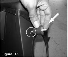
Attach the vibra mount to the outside of the heat shield and secure.
