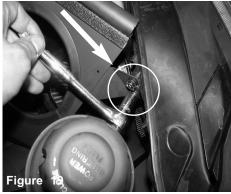
Secure the tab using the bolts from step 11. Secure and tighten using 10mm socket and ratchet.
