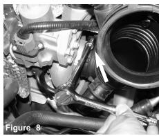
Loosen the clamp on the turbo using 10mm socket and ratchet.
