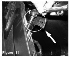
Loosen the 2 bolts holding in the air box bracket located behind headlight. Save the 2 screws for later install. Remove the bracket.
