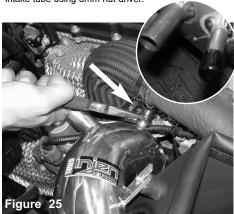
Connect the Crank case line and secure. Auto trans, cap off 3/8" fitting on intake tube using provided vinyl cap. Connect brake booster line( manual trans only)
