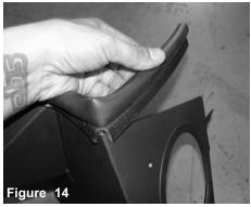
Attach the rubber trim to the top of the heat shield. You can cut a notch into the corner if necessary for easier installation.
