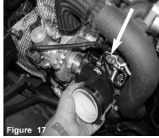
Install the 90degree hose with clamps provided to the turbo. Install 2-1/2 side to the turbo. Position clamps for easy access. Do not TIGHTEN!
