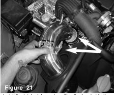
Install the intake tube and position the bracket to the vibra mount and tube to the hose.
