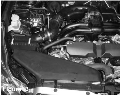
Figure 3 Stock box shown in this picture. Disconnect battery before the install.
