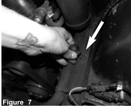
Figure 4 With 10 mm socket, loosen the screw holding in the temperature sensor and pull back.
