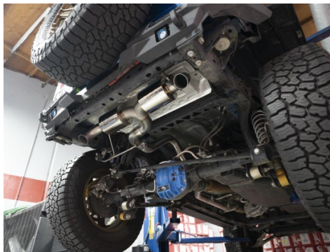
20. Ensure all bolts and clamps are properly secured.
