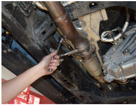
2. Remove the two nuts securing the mid pipe to the flex pipe. Then detach the front hanger from the rubber insulator.
