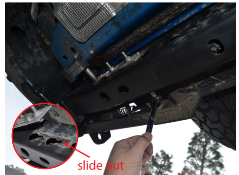
9. 2.3L MODELS ONLY: Remove the OEM hanger by loosening the two bolts and then sliding it out. The bolts can be accessed from the rear of the subframe.
