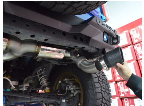
18. OPTIONAL: Attach exhaust tips to the tip extension.
