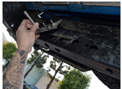
12. 2.3L MODELS ONLY: Slide the Injen hanger bracket into place. Then secure the two bolts.
