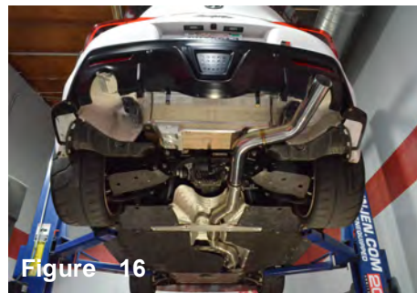
Figure 13 Make sure the mid pipe hanger is straight on isolator.
