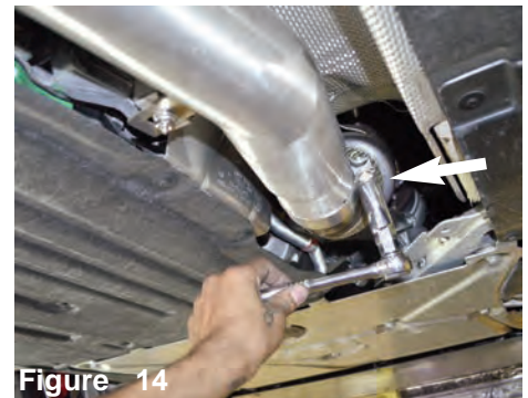
Figure 11 install the rear-section and secure using V band clamps. Do not tighten. place exhaust hanger to the rubber isolator. Note: Exhaust system has room for adjustment, reposition and tighten for best fit.
