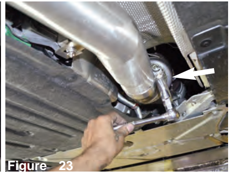
Figure 23 Once completed adjustment and clearance, tighten all clamps using 17mm and 13mm. Re-adjust and reposition if necessary.
