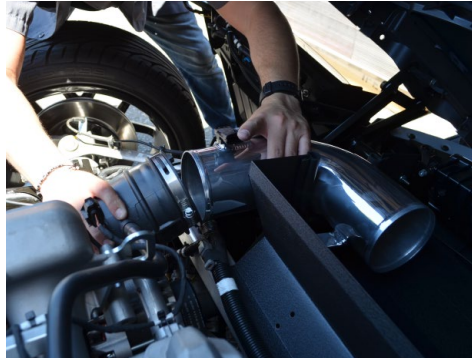
17. Insert the injen tube into the OEM hose. Leave the OEM clamp loose for now.
