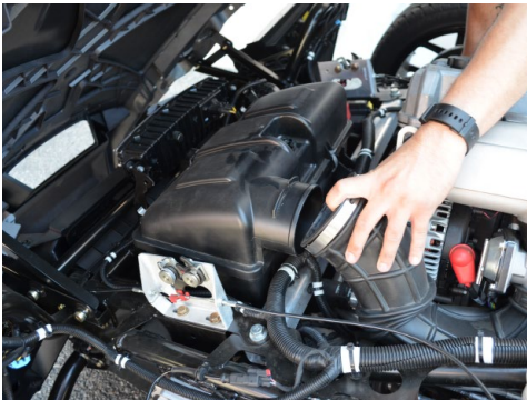
4. Loosen the clamp holding the intake hose to the air box and detach the intake hose from the air box.
