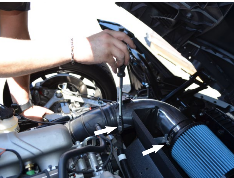
19. Install the air filter onto the intake tube, then secure the filter clamp and the OEM hose clamp.
