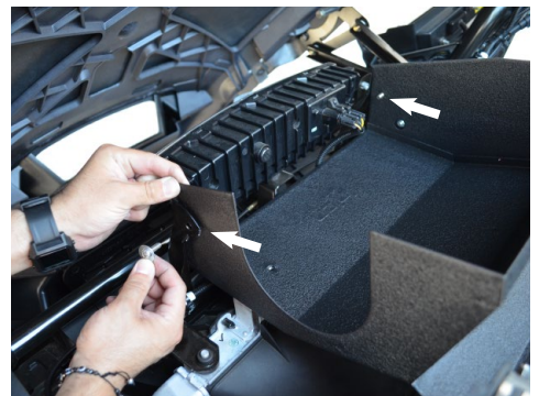
12. . Install the provided M6X20mm bolt onto the driver side of the heat shield. Secure both bolts with M6 nut and washer.
