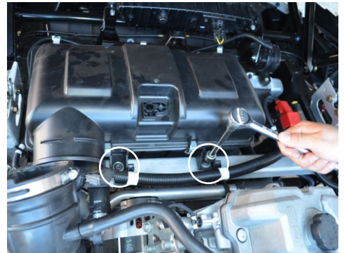
6. Remove the two bolts holding down the back of the air box.
