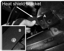
**14.** A)Now install the bracket on heat shield to the front clip located on fire wall. Make sure bracket sits under clip. Secure using provided M6 socket cap screw and fender washer. B)Secure the stand off stud using provided M6 nut and fender washer.
