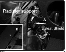
**13.** A)Install the heatshield into the vehicle and position bracket to the front radiator support. Secure using bolt from step 9. Tighten and secure. B)Now install the bottom of the heat shield hole to the stand off stud.
