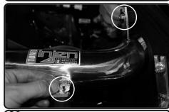
**23.** Secure the brackets using provided M6 nuts and fender washers.
