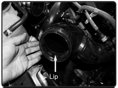
**16.** Now install the 4" elbow with clamps provided to the large turbo housing side. Make sure the side with no lip is installed on the housing. Position like image above.
