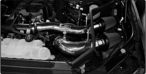
Congratulations! You have just completed the installation of this intake system. Periodically, check the alignment of the intake, normal wear and tear can cause nuts and bolts to come loose. Note: Check clearance and adjust if needed! Failure to check the alignment and adjust the intake can cause damage that will void the warranty. Injen Technology is not responsible for any damages caused by/from improper installation.
