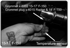
**26.** 15-17' F150 only install grommet x-8002 to the hole on 3.5" tube. Now install the temperature sensor to grommet and secure. Reconnect the harness to the temperature sensor. *Install the x-6015 grommet to 3" tube.*
