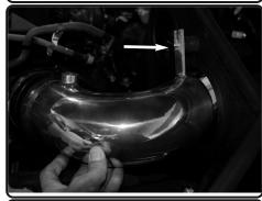
**19.** Position for the best fit, make sure the elbow fits in the natural position for best fit and clearance. *Note:see last page for crankcase tube installation.*
