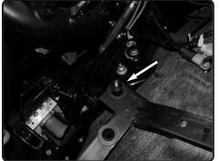
**12.** Locate the stock air box grommet in above image. Install the stand off stud to the grommet and secure.
