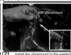
**21.** Install the vibramount to the welded fitting on intake tube, secure the vibramount and tighten.
