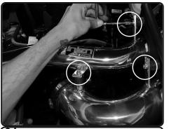
**24.** Tighten all the vibramounts using 10mm socket and ratchet.
