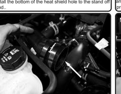
**17.** Install the 3" straight hose with clamps provided to the secondary turbo housing. Tighten the clamp on housing only using 8mm nut driver.
