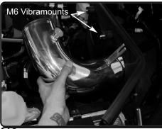
**18.** Install two vibramount to the thredded inserts on heat shield. Install the large intake pipe, make sure the 3.5" side goes through heat shield. Position the bracket to the vibramount and tube to 4" elbow. Do not tighten.
