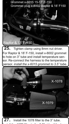
**L** Install the 1078 filter to the 3" tube. Install the 1079 filter to the 3.5" side of the large tube. Tighten clamps using 8mm nut driver.
