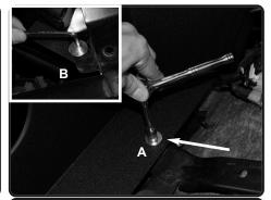
**15.** A)Now secure and tighten using 10mm socket and ratchet. B)Secure the bracket using allen key.
