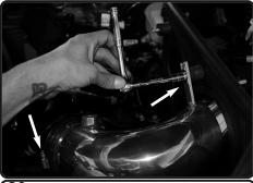
**20.** Secure the bracket using provided m6 nut and fender washer tighten using 10mm socket and ratchet. Tighten clamps using 8mm nut driver. Page 4 PF9015
