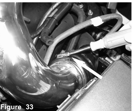
Figure 34 Re-connect the temperature sensor harness.
