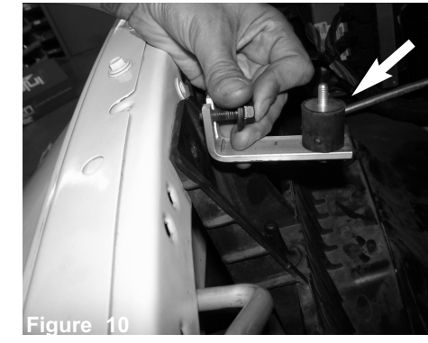
Figure 11 Install the bracket p/n: x-20091 to the spot where the bolt was removed and reuse the bolt removed from figure 8 to secure the bracket to the fender well. Install the vibramount, nut and washer to the bracket.
