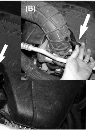
Figure 6(B) Firmly pull air temp sensor out of factory air duct. This sensor will be re-used later.
