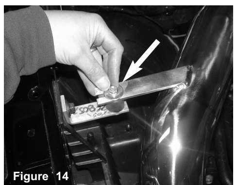
Figure 15 Place a M6 nut and fender washer onto the bracket to secure it to the vibramount
