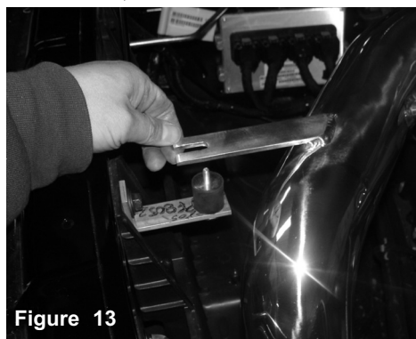
Figure 14 Align the bracket onto the vibramount
