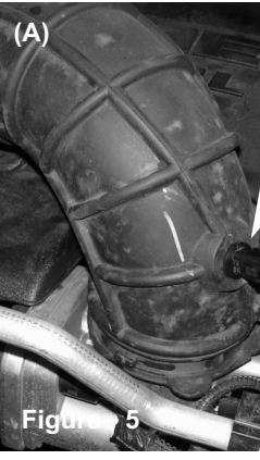
Figure 6(A) Air temp sensor with harness removed
