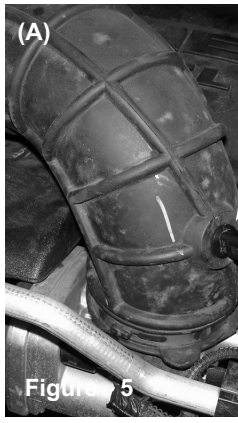
Figure 5 (A) Air temp sensor with harness removed Figure 5 (B) Firmly pull air temp sensor out of factory air duct. This sensor will be re-used later.
