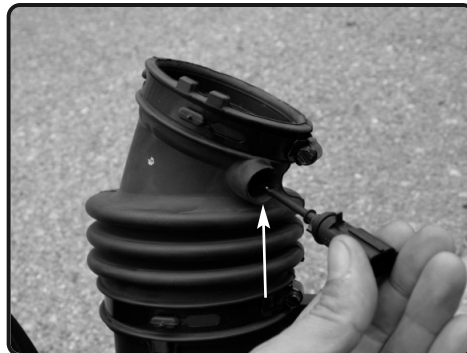
6. Now carefully remove the temperature sensor from the intake tube.
