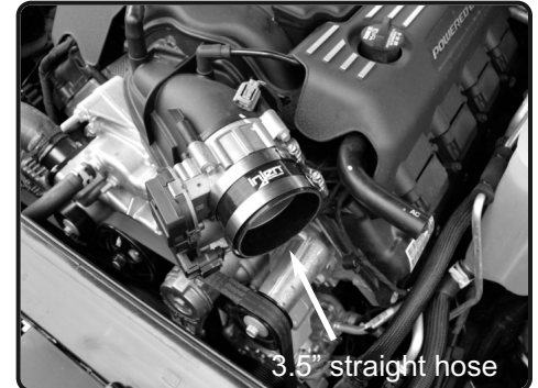
7. Install the 3.5" straight hose to the throttle body. Tighten clamp on throttle body using 8mm nut driver.
