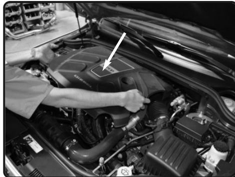
2. Lift firmly on the engine cover and temporarily remove from the engine bay for now.
