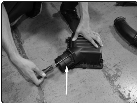
5. Unbolt the MAF sensor from the O.E. upper air box assembly. This MAF sensor will be reused in this intake system.
