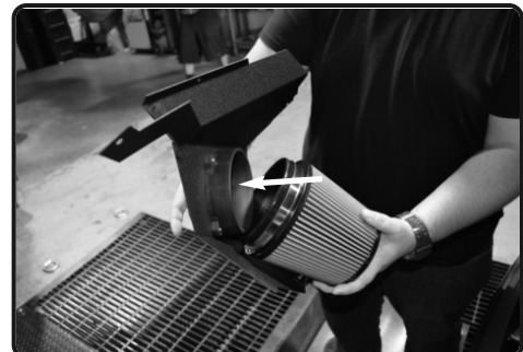
11. Place the filter onto the velocity stack and then secure the clamp.
