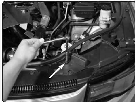
6. Temporarily remove this 10mm bolt from the radiator support. This bolt will secure the Injen heatshield to the radiator support later in figure 12 .
