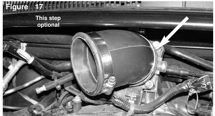
Figure 17 This step optional Position the hose so that it does not hit the support brace.
