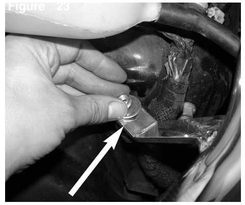
Secure the bracket using M6 nut and washer.
