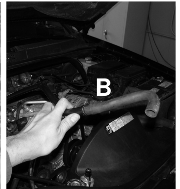
Figure 10 Lift up the bottom half of the air box
