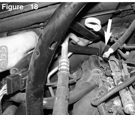
Figure 18 Install the new provided 15mm hose to the fitting on engine side.
