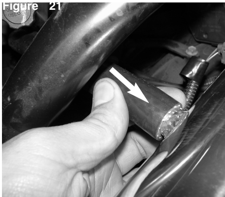
Attach the other end of the 15mm hose to the fitting on the intake tube.
