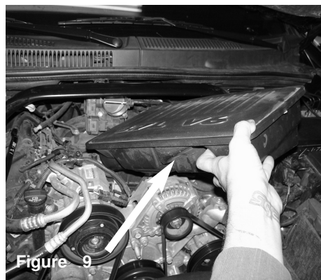
Figure 10 Lift up the bottom half of the air box
