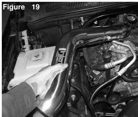
Figure 19 Position the intake tube to the elbow hose and bracket to the vibra mount.
