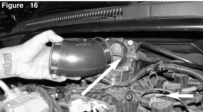
Figure 16 Install the 2-3/4" side of elbow hose with clamps provided to the throttle body.
