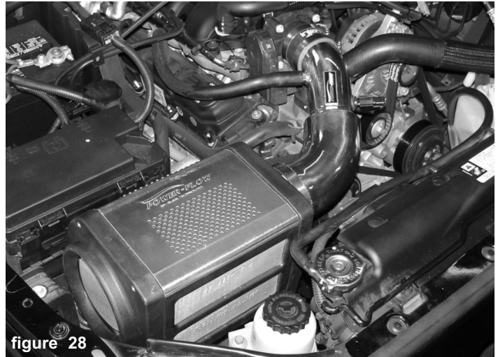
figure 28 Periodically, check the entire air intake system for any possible movement. Normal wear and tear can cause clamps and hoses to loosen over time, periodic adjustments to the intake system will enhance the life of your intake and prevent your warranty to become null and void.
