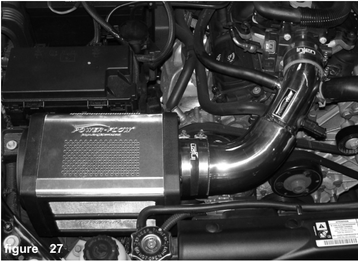
figure 27 Check the entire air intake system for any air leaks, rattling or any loose clamps and hoses before starting the engine. Once you have checked the entire system, start the engine and let it idle for 5 to 10 minutes. Allow the on-board computer to adjust to the added volume of air prior to driving.
