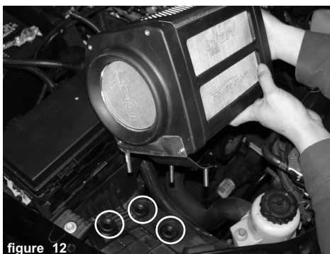
figure 12 Once the bracket has been installed, continue to lower the entire power box in the the engine compartment. The three metal pegs are aligned to the stock grommets and plugged into the grommets. Page 2 of Part# PF5002
