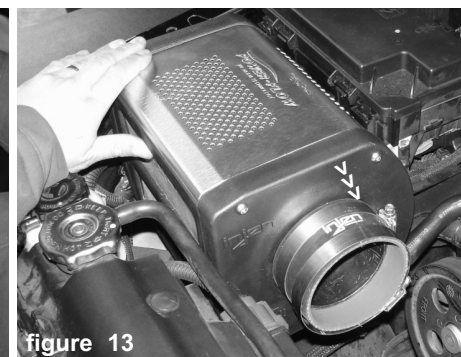
figure 13 The three metal pegs are aligned and pressed into the stock grommets. The 3 3/4" straight hose is pressed over the the velocity stack. Two power bands are used on the hose. The clamp on the velocity stack is now tightened.
