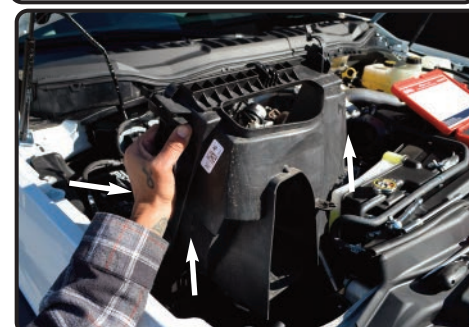
10. Now carefully lift up and remove the bottom half of the air box out of the vehicle.
