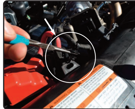
3. With a prying tool, pull back the harness clip away from the air box.
