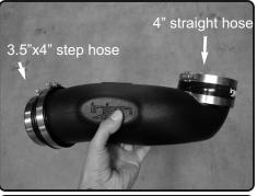
**18.** Install the the 3.5"x4" straight hoses to the tube with clamps provided.
