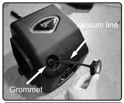
1. Connect the 3mm vacuum line to the Filter Monitor. Place the grommet into the 3/4" in the air box. Then run the 3mm vacuum line through the grommet.
