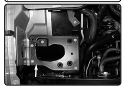
**9.** Leave the OEM bracket in vehicle. this will be used for new intake system.
