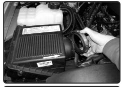
**5.** Loosen the clamp using 8mm nut driver. Remove the MAF sensor from air box. Remove the factory coupler from MAF sensor.
