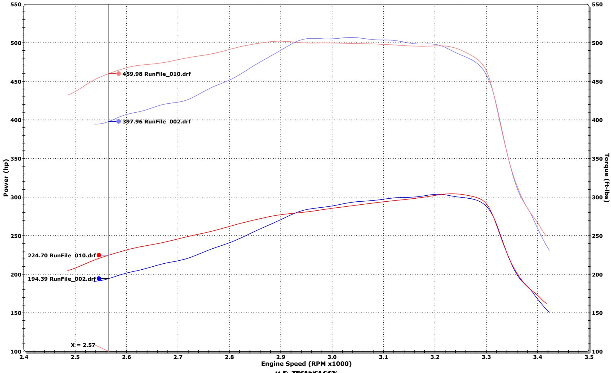
■ RunFile\_002.drf - 5/2/2014 11:43:00 AM Run Type: RO Run Conditions: 93.15 °F, 29.16 in-Hg, Humidity: 24%, SAE: 1.04
